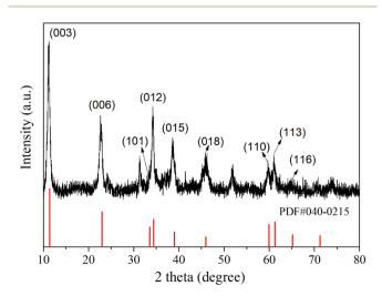
Fig. 1 XRD characterization of synthesized layered double hydroxides.
