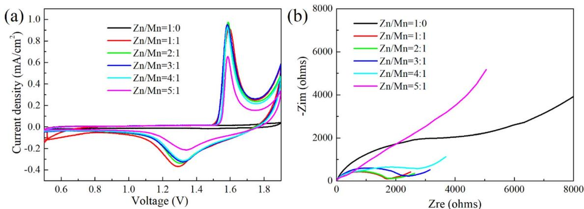
Fig. 6 (a) Cyclic voltammetry (CV) at a scan rate of  $1 \text{ mV s}^{-1}$  (b) electrochemical impedance spectroscopy (EIS) at a frequency range from  $10^5$  to  $0.1 \text{ Hz}$  in analysis of Zn–Mn batteries based on LDHs substrate with varying Zn to Mn molar ratios in the electrolyte.
