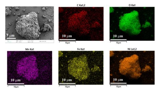
Fig. 2 SEM-EDS characterization of synthesized layered double hydroxides.
