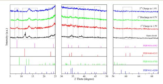
Fig. 7 Ex situ X-ray diffraction (XRD) analysis of Zn-Mn batteries with an LDHs substrate and a Zn/Mn molar ratio of 4:1 in the electrolyte under different charge-discharge states.
