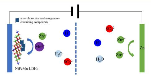
Fig. 10 The schematic illustration of the mechanism for the Zn-Mn reversible deposition battery based on LDHs.
