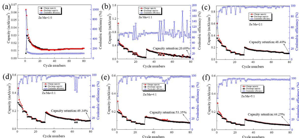
Fig. 5 Rate capability and cycling stability of Zn–Mn batteries based on LDHs substrate with varying Zn to Mn molar ratios in the electrolyte (a) Zn : Mn = 1 : 0 (b) Zn : Mn = 1 : 1 (c) Zn : Mn = 2 : 1 (d) Zn : Mn = 3 : 1 (e) Zn : Mn = 4 : 1 (f) Zn : Mn = 5 : 1.
