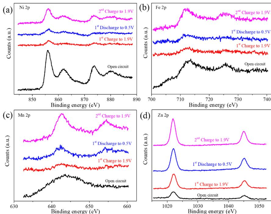
Fig. 9 *Ex situ* X-ray photoelectron spectroscopy (XPS) analysis of Zn–Mn batteries with an LDHs substrate and a Zn/Mn molar ratio of 4 : 1 in the electrolyte under different charge–discharge states. (a) Ni 2p (b) Fe 2p (c) Mn 2p (d) Zn 2p.
