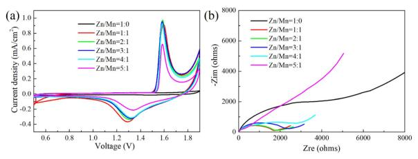
Fig. 6 (a) Cyclic voltammetry (CV) at a scan rate of 1 mV s<sup>-1</sup> (b) electrochemical impedance spectroscopy (EIS) at a frequency range from  $10^5$  to 0.1 Hz in analysis of Zn-Mn batteries based on LDHs substrate with varying Zn to Mn molar ratios in the electrolyte.
