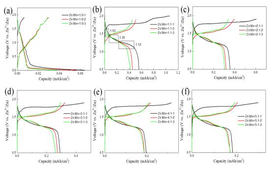
Fig. 4 Charge and discharge curves of Zn-Mn batteries based on LDHs substrate with varying Zn to Mn molar ratios in the electrolyte at a current of 0.2 mA. (a) Zn : Mn = 1 : 0 (b) Zn : Mn = 1 : 1 (c) Zn : Mn = 2 : 1 (d) Zn : Mn = 3 : 1 (e) Zn : Mn = 4 : 1 (f) Zn : Mn = 5 : 1
