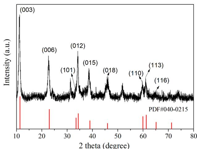
Fig. 1 XRD characterization of synthesized layered double hydroxides.
