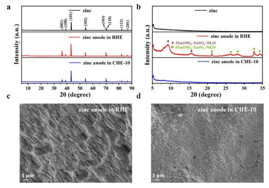
Fig. 6 Characterization of the anodes: (a) XRD patterns of zinc anodes of batteries using the RHE and CHE-10 after 1000 cycles at 1.5 A g<sup>-1</sup>. (b) Partial enlarged views ( $2\theta = 5-35^{\circ}$ ) of the XRD patterns. SEM images of the corresponding zinc anodes of batteries using (c) RHE and (d) CHE-10 after 1000 cycles at 1.5 A g<sup>-1</sup>.
