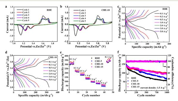
Fig. 4 Electrochemical performance of batteries using different electrolytes: (a and b) cyclic voltammograms. (c and d) Charge/discharge profiles. (e) Rate performance. (f) Cycling performance.
