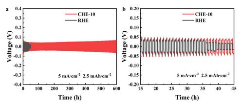
Fig. 5 (a) Polarization curves of Zn//Zn symmetric batteries using RHE and CHE-10. (b) Enlarged voltage profiles of 15 to 45 h.
