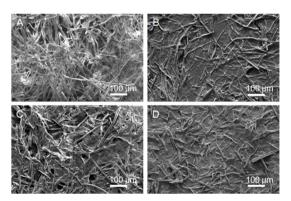
Fig. 1 FE-SEM images showing pulp fibre structure (A) before acidic treatment and the transformed structures after acidic treatment at 6, 12, and 24 hours (B, C, and D, respectively).
