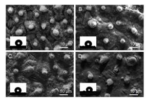
Fig. 4 FE-SEM images of lotus-leaf surface sprayed with 1.5% w/v colloidal cellulose for (A) 0, (B) 10, (C) 20 and 30 (D) seconds, with inset digital images showing the DI water contact angle for each configuration.
