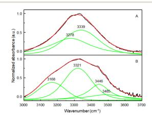
Fig. 6 FT-IR spectra of (A) pulp fibre and (B) cellulose film with Voigt curve fitting in the range of  $3000-3700~\rm{cm}^{-1}$ .
