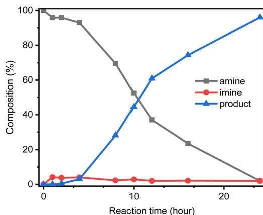
Fig. 8 Reaction progress of *N*-alkylation of aniline. Aniline (1 mmol) react with benzyl alcohol (2 mmol), and catalyst GSOIC/TMPP (0.002 g/0.006 mmol); composition distribution of nitrogen-containing products was determined by GC-MS.
