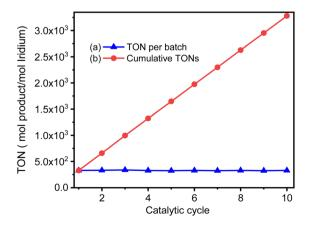
Fig. 11 The TON of the catalytic cycles for the transformation of aniline into N-benzylaniline; (a) TON of each cycle, (b) accumulated TON, for the cycle n the accumulated TON was calculated by  $TON_n^{acc} = \sum_{k=1}^n x_k$ .
