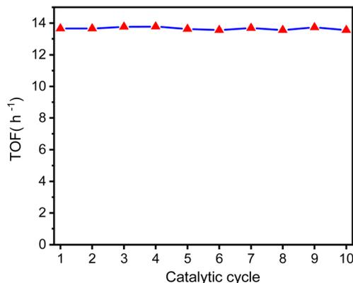
Fig. 10 The TOF of the catalytic cycle of converting aniline into *N*-benzylaniline shows that the catalytic ability of the GSOIC/TMPP catalytic system for the hydrogen borrowing reaction is quite stable.
