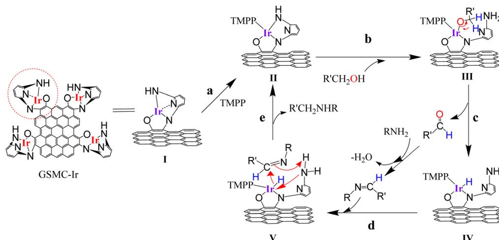
Scheme 4 A plausible mechanism for C–N bond formation in the GSOIC/AL catalytic systems.
