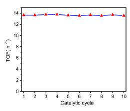
Fig. 10 The TOF of the catalytic cycle of converting aniline into *N*-benzylaniline shows that the catalytic ability of the GSOIC/TMPP catalytic system for the hydrogen borrowing reaction is quite stable.
