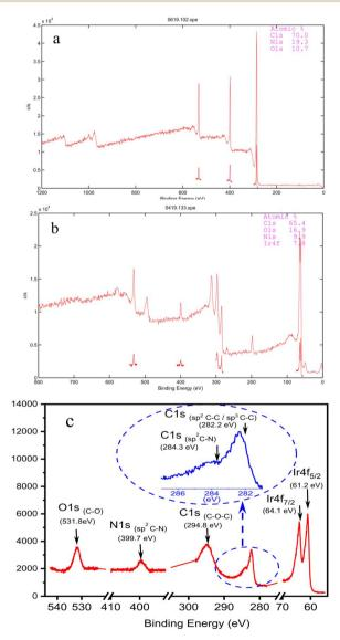
Fig. 3 (a) Survey XPS of GODAP; (b) survey XPS of GSOIC; (c) chemical states of elements in GSOIC
