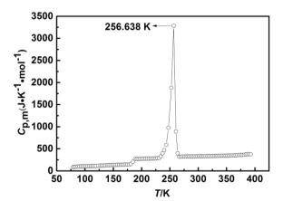
Fig. 3 The experimental molar heat capacities in Table 2 of [ $C_2$ 2O2IM] [SCN] in the temperature range from 79 to 393 K.
