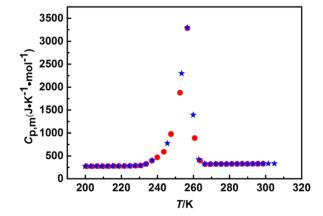
Fig. 4 Two series of experimental molar heat capacities of  $[C_22O2IM]$  [SCN] in the fusion region( $\bullet$  red solid circle is the first series,  $\star$  blue solid pentacle is the second series).
