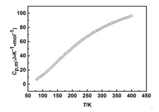
Fig. 2 The heat capacities of  $\alpha$ -Al<sub>2</sub>O<sub>3</sub> in the temperature range from 78 to 400 K.
