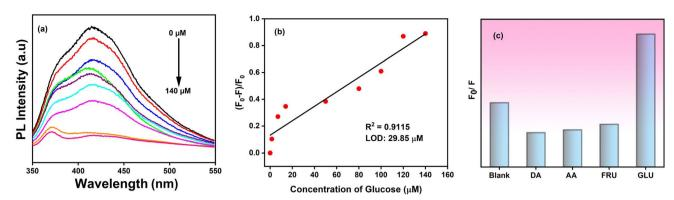
Fig. 3 (a) The emission spectra values of *versus* concentration of glucose  $0-140 \mu M$ , (b) linear calibration of the fluorescence intensity ratio (( $F-F_0$ )/ $F_0$ ) and LOD value, (c) the graph of the selectivity test of the sensor towards different biomolecules (blank, DA, AA, FRU, GLU).
