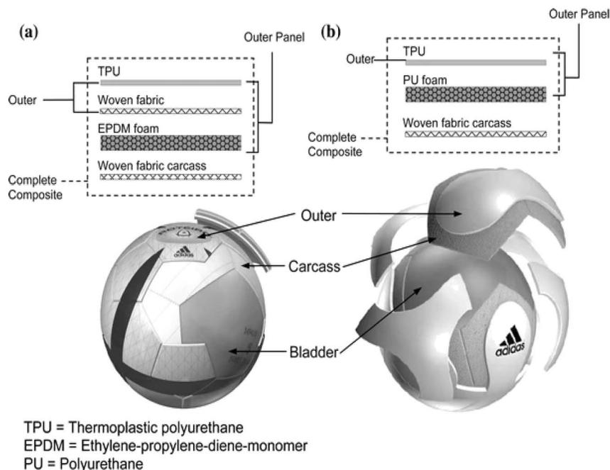
Fig. 4 (a and b) Soccer balls are based on multi-layer textile-reinforced polymer composites.<sup>55</sup> Copyright 2008, Springer.
