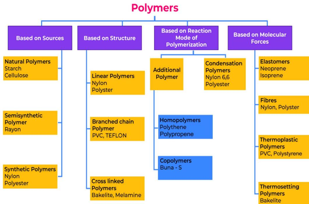
Fig. 6 The classification of polymers is illustrated in the chart below.<sup>64–68</sup>
