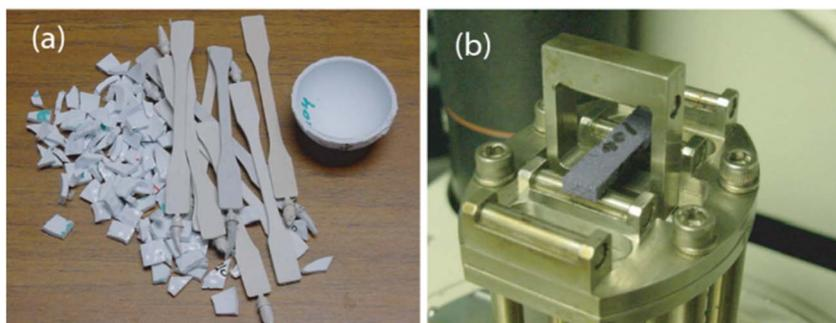
Fig. 10 (a) Calibration ball cover, cover material, and tensile test specimens, (b) core flexure specimen in a 3-point bend DMA fixture.<sup>170</sup>
