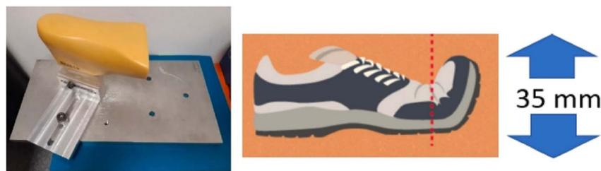
Fig. 11 The setup used for the stiffness test. A stiffness test was performed using the Instron 3360 universal testing machine. Footwear was tested with no insole. Distance of extension – 35 mm.<sup>161</sup> Copyright 2022, Elsevier.
