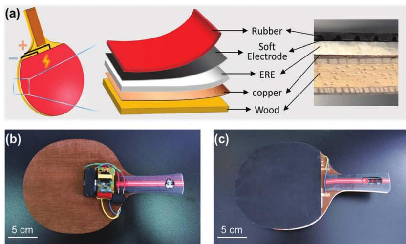
Fig. 9 (a–c) Schematic illustration of smart table tennis racket based on anisotropic electrorheological elastomers (EREs).<sup>176</sup> Copyright 2021, Wiley.
