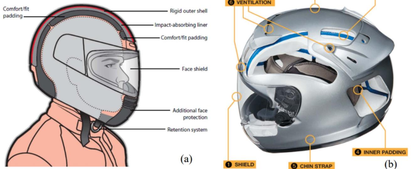
Fig. 7 Schematic diagrams showing the various components in a (a) typical motorcycle helmet and (b) a Shoei motorcycle helmet.<sup>71</sup>
