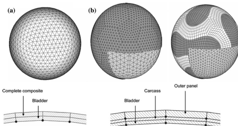
Fig. 12 (a and b) Composite soccer balls with multi-layer textile-reinforced polymer composites with high viscoelasticity.<sup>55</sup> Copyright 2008, Springer.
