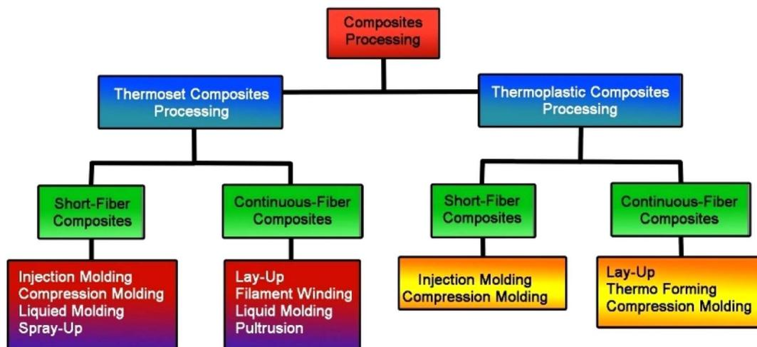
Fig. 8 Fabrication procedures of various polymer matrix composites.
