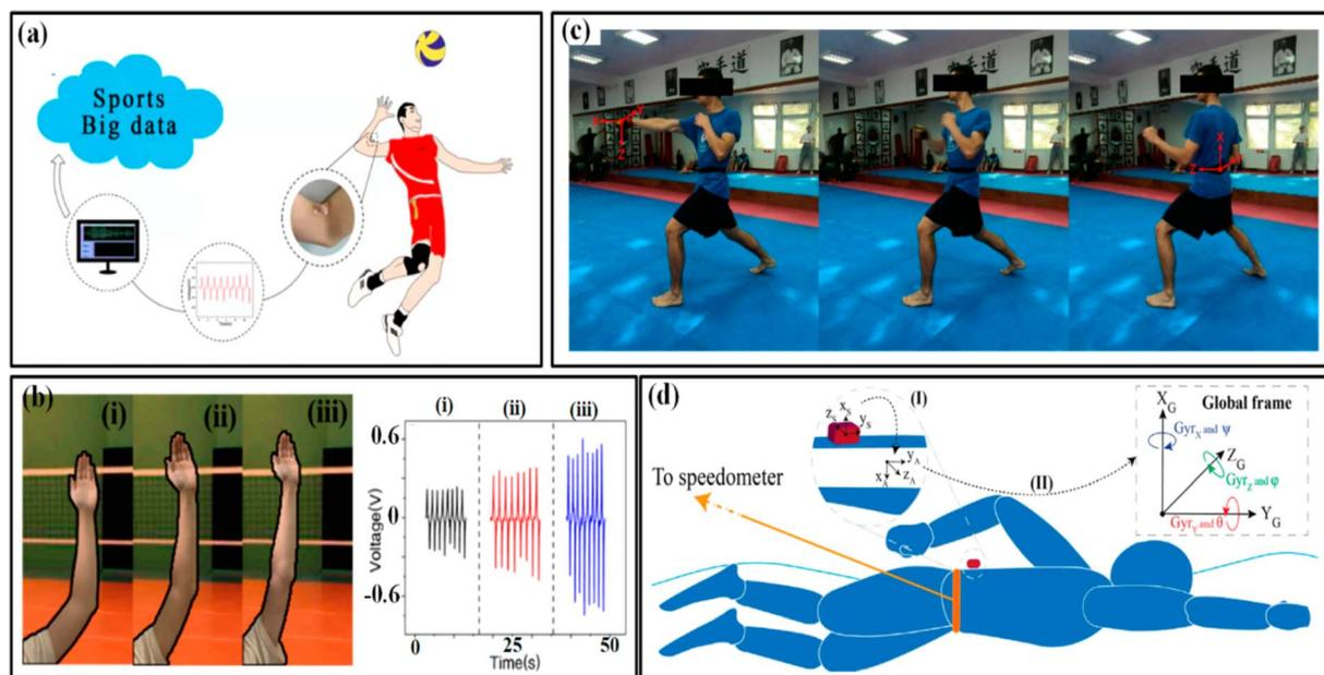
Fig. 17 The kinematic markers in the trunk and limb are (a) the elbow bending angles in volleyball and (b) the observed outcomes of three elbow bending states (i–iii).<sup>184</sup> Copyright 2021, MDPI. (c) Karate's use of IMUs. (d) Using IMUs while swimming.<sup>185</sup> Copyright 2021, Frontiers in Bioengineering and Biotechnology.
