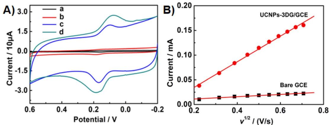
Fig. 2 (A) CVs of Bn at different electrode surfaces: bare GCE (a), UCNPs/GCE (b), 3DG/GCE (c) and UCNPs-3DG/GCE (d) in 0.1 M PBS (pH = 7.0). Scan rate:  $0.1 \text{ V s}^{-1}$ . (B) Relationship between the anodic peak current and the square root of the scan rate for different electrodes in 0.1 M KCl solution containing  $1.0 \text{ mM K}_3\text{Fe}(\text{CN})_6$ .
