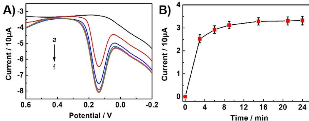
Fig. 4 (A) DPVs of Bn at the UCNPs-3DG/GCE at different accumulation times in 0.1 M PBS ( $\text{pH} = 7.0$ ). The concentration of Bn:  $5.0 \times 10^{-6} \text{ mol L}^{-1}$ . (B) The oxidation peak current of Bn vs. the accumulation time: (a) 0 min, (b) 3.0 min, (c) 9.0 min, (d) 15.0 min, (e) 21.0 min, and (f) 24.0 min.
