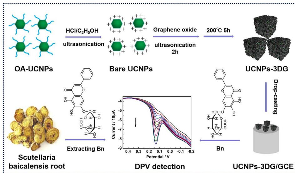
Scheme 2 Fabrication process of UCNP-3DG and its application in electrochemical detection of Bn in natural plant samples.
