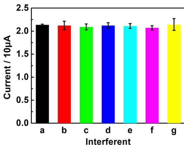
Fig. 9 DPV responses of the UCNPs-3DG/GCE to Bn in the presence of various interfering substances. (a) No interfering substance, (b)  $\text{Zn}^{2+}$ , (c)  $\text{Mg}^{2+}$ , (d) Suc, (e) Glu, (f) L-cys, and (g) Ea.  $c_{\text{Bn}} = 2.0 \times 10^{-6}$  M.
