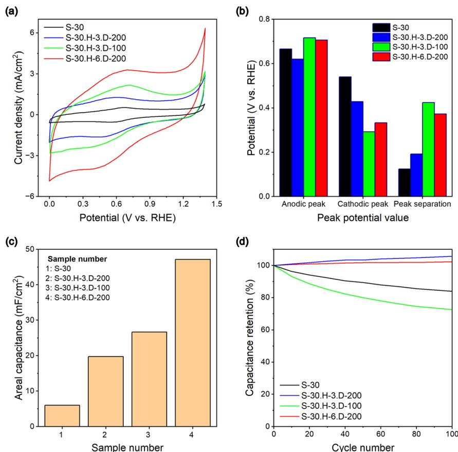
Fig. 9 Cyclic voltammograms (a), peak potential (b), area capacitance (c), and capacitance retention (d) of the fabricated samples at a  $50 \text{ mV s}^{-1}$  scan rate in  $0.5 \text{ N H}_2\text{SO}_4$  electrolyte.
