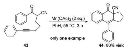
Scheme 14 Synthesis of ADHNs via manganese(III)-catalyzed oxidative cyclization of aryl 1-cyanoalk-5-ynyl ketone.
