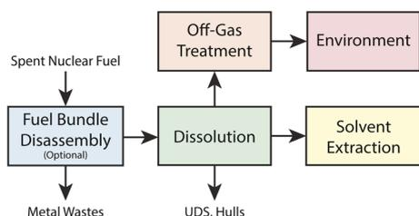
**Fig. 1** Schematic of process steps that are covered in this review. Fuel bundle disassembly is covered in Section 2, dissolution and off gas treatment in Section 3, solvent extraction in Section 4, and environment in Section 5.
