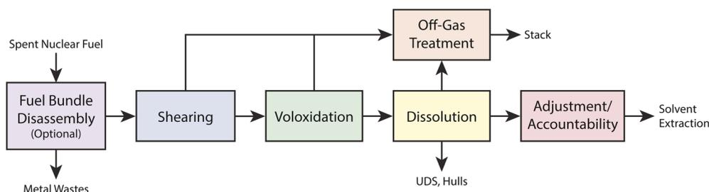
Fig. 2 Block flow diagram for aqueous head-end processing.<sup>10</sup> This figure was reprinted with permission. Copyright 2008 CRESP.
