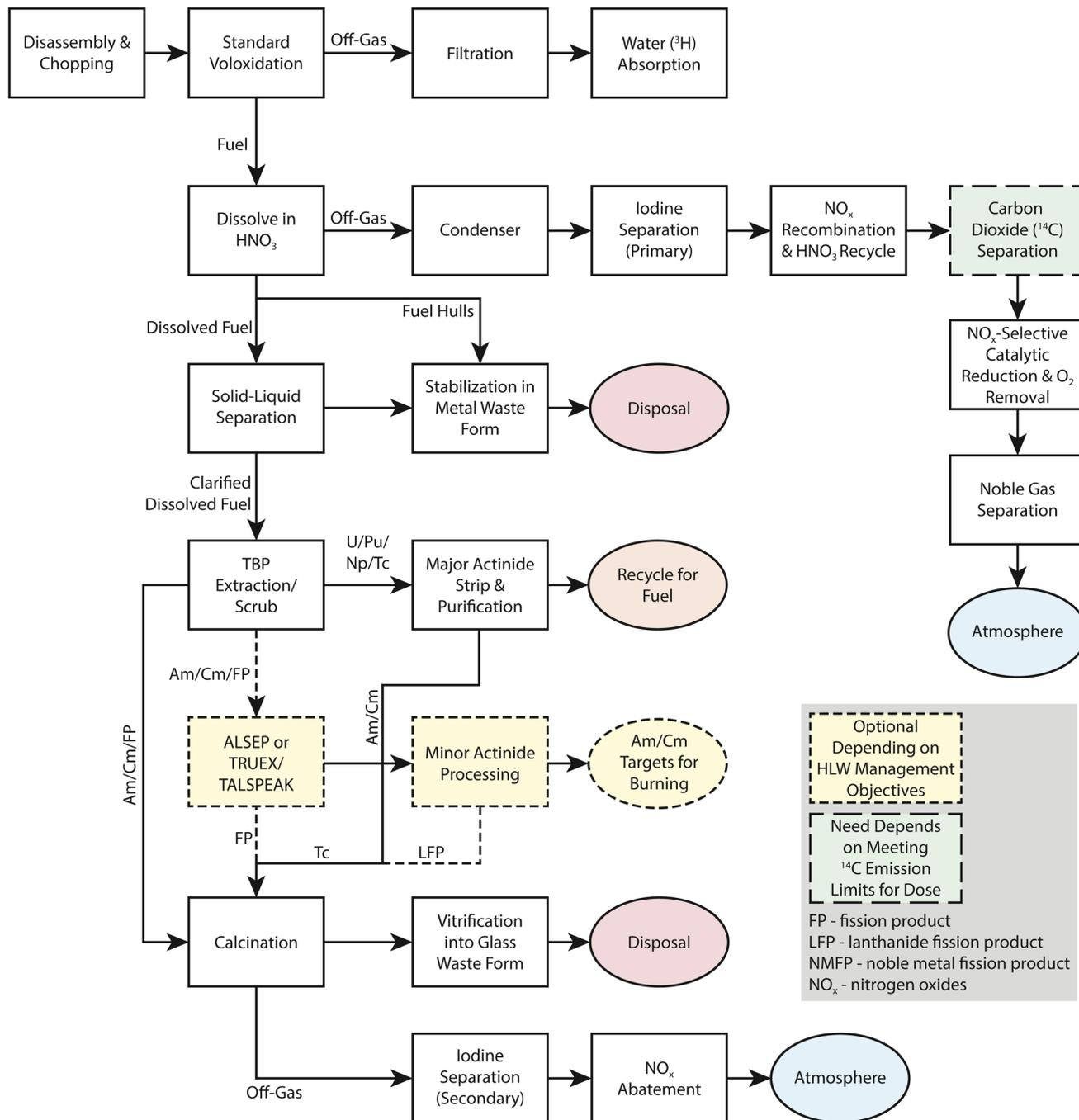
Fig. 5 Basis of comparison flowsheet for UNF actinide recovery. This figure was recreated with permission from Arm.<sup>79</sup>
