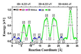
Fig. 4 Energy vs. reaction coordinate profile of the Na<sub>2</sub>Mg<sub>3</sub>Cl<sub>8</sub> structure derived from BV computations.
