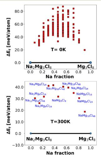
Fig. 3 Formation energies of pseudo-binary phases of  $Na_2Mg_3Cl_8$  at 0 (top) and 300 K (bottom). The red point represents the unstable phases in  $Na^+$  vacancy generation.
