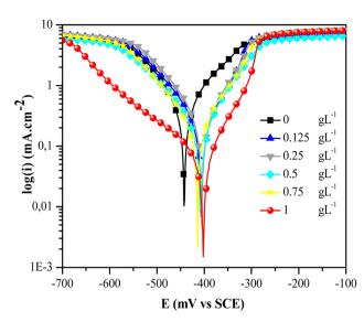
Fig. 3 Semi-logarithmic polarization curves of the steel sample in 0.5 M HCl at various inhibitor concentrations.
