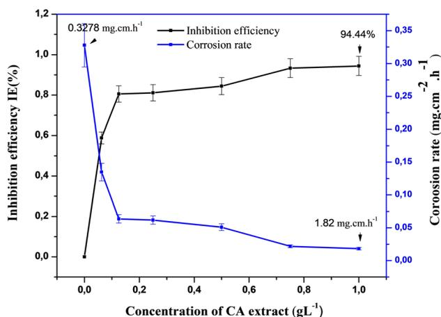
Fig. 2 Corrosion rate and inhibition efficiency variation with the increasing concentration of CA extract.
