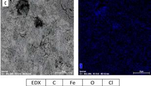
Fig. 7 SEM and EDX data for C45 steel samples: (A) polished, (B) with 0.5 M HCl, (C) with 0.5 M HCl + 1 g  $\rm L^{-1}$  of CA extract.
