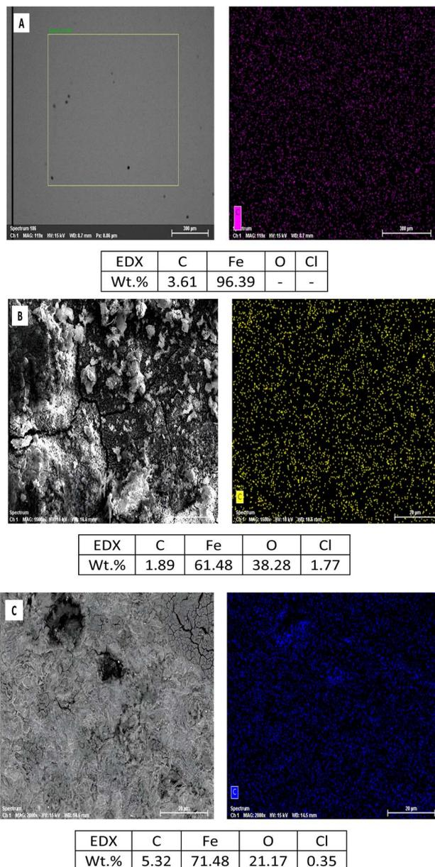
Fig. 7 SEM and EDX data for C45 steel samples: (A) polished, (B) with 0.5 M HCl, (C) with 0.5 M HCl + 1 g L<sup>-1</sup> of CA extract.
