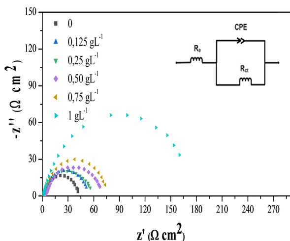
Fig. 5 Nyquist diagrams of the steel samples in  $0.5 \text{ M HCl}$  at different concentrations of CA extract; inset shows the equivalent electrical circuit fitting the experimental data.
