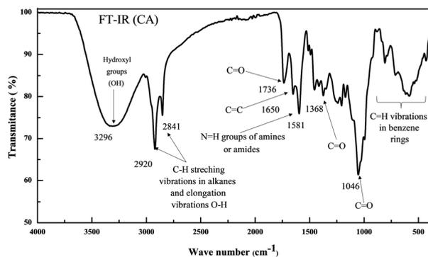
Fig. 1 FTIR (ATR) spectrum of the (CA) extract.
