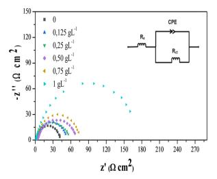
Fig. 5 Nyquist diagrams of the steel samples in 0.5 M HCl at different concentrations of CA extract; inset shows the equivalent electrical circuit fitting the experimental data.
