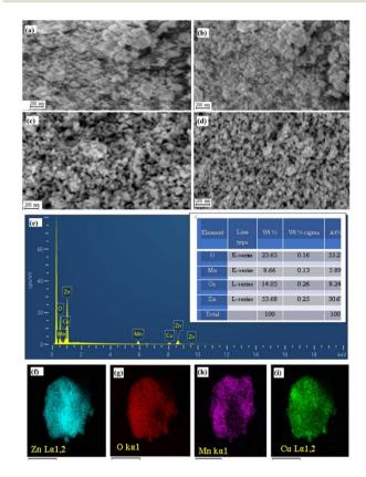
Fig. 3 SEM image of (a) Z; (b) M; (c) C; and (d) MZC. (e) EDS elemental composition; and Elemental mapping of (f) Zn; (g) O; (h) Mn; and (i) Cu.
