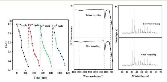
Fig. 11 (a) Reusability of the MZC nanocomposite photocatalyst after four successive runs; (b) FTIR spectra of the MZC nanocomposite before and after recycling; (c) XRD diffraction of the MZC nanocomposite before and after recycling.
