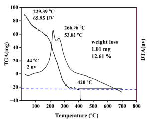
Fig. 1 Thermal analysis of the MZC heterojunction nanocomposites
