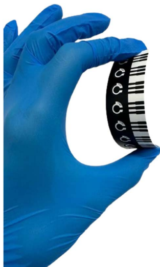
Fig. 4 Screen-printed sensors produced on flexible substrate.
