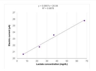
Fig. 11 Evaluation of plasma sample on SPE-C/G-RE-Nafion-LOx sensors. Each point on the graph represents the average oxidation current obtained in each evaluated biological sample, and the average was calculated based on triplicate tests. 6.3 mg dL $^{-1}=(20.64\pm6.13)$   $\mu\text{A}, 22.5$  mg dL $^{-1}=(21.76\pm3.73)$   $\mu\text{A}, 36.9$  mg dL $^{-1}=(23.57\pm3.54)$   $\mu\text{A}$  and 67.6 mg dL $^{-1}=(25.77\pm3.23)$   $\mu\text{A}.$
