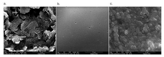
Fig. 6 Images of the stages of lactate biosensor production with  $10\,000\times$  original magnification: (a) unmodified WE, (b) WE modified with a Nafion polymeric film, and (c) WE modified with Nafion and LOx.
