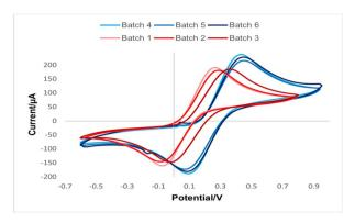
Fig. 5 CV for SPE-C/G-RE (Process 1, red line) and SPE-Ag/AgCl-RE (Process 2, blue line) in potassium ferrocyanide (10 mol  $L^{-1}$ ) and potassium chloride (1 mol  $L^{-1}$ ) at scan rate 100 mV. The voltammograms resulted from the average of 10 measurements in each batch.
