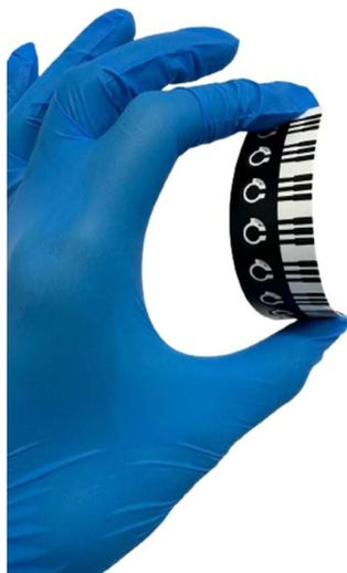
Fig. 4 Screen-printed sensors produced on flexible substrate.
