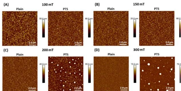
Fig. 4 10  $\mu\text{m} \times 10 \mu\text{m}$  AFM scans of oCVD PT films deposited on plain and PTS substrates at different deposition pressures, including (A) 100 mT, (B) 150 mT, (C) 200 mT, and (D) 300 mT.
