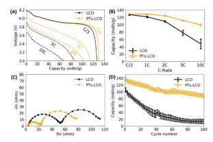
Fig. 5 The effect of oCVD PT coating on the electrochemical performance of LiCoO $_2$ . (A) The comparison of discharge curves at different C-rates for the two LiCoO $_2$  electrodes. (B) Statistical comparison of cell capacities (four samples) at different C-rates tested at 3.0-4.2 V. (C) The comparison of electrochemical impedance spectroscopy of the two types of coin cells measured at 4.0 V. (D) Capacity degradation of LiCoO $_2$  electrodes tested at 5C in the voltage range of 3.0-4.5 V.
