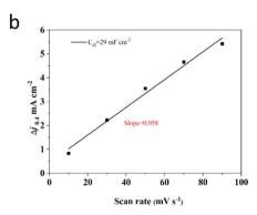
Fig. 8 (a) CVs of Ni-10.84 wt% Mo tested in a non-faradaic region of the voltammogram in 1 M KOH at different rates from 10 to 90 mV s<sup>-1</sup>. (b) The corresponding capacitive current at 0.40 vs. SCE as a function of scan rate for as-deposited samples
