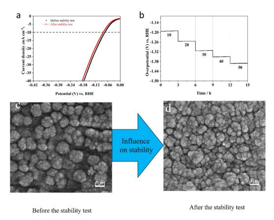
Fig. 9 Initial LSV curves and after 1000 CV cycles (a) and *E*-*t* curves at different current densities (b) measured for Ni–Mo films in 1 M KOH containing 10.84 wt% Mo. SEM image before (c) and after (d) the stability test.
