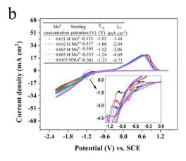
Fig. 2 Cyclic voltammograms of different  $Ni^{2+}$  contents in the EG + 0.15 M H<sub>3</sub>Cit system with 0.084 M Mo<sup>6+</sup> (a) and Mo<sup>6+</sup> contents in the EG + 0.15 M H<sub>3</sub>Cit system with 0.30 M  $Ni^{2+}$  (b) measured on a glassy carbon electrode with a scan rate of 50 mV s<sup>-1</sup> at 323 K.
