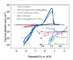
Fig. 1 Cyclic voltammograms of the EG + 0.15 M H<sub>3</sub>Cit system (curve 1), EG + 0.15 M H<sub>3</sub>Cit system with 0.084 M Mo<sup>6+</sup> (curve 2), EG + 0.15 M H<sub>3</sub>Cit system with 0.30 M Ni<sup>2+</sup> (curve 3) and EG + 0.15 M H<sub>3</sub>Cit system with 0.084 M Mo<sup>6+</sup> + 0.30 M Ni<sup>2+</sup> (curve 4) measured on a glassy carbon electrode with a scan rate of 50 mV s<sup>-1</sup> at 323 K.
