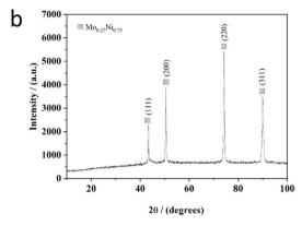
Fig. 3 EDS (a) and XRD (b) pattern of Ni–Mo alloy films obtained from the EG system at 333 K for 20 min, including 0.30 M Ni<sup>2+</sup> and 0.084 M Mo<sup>6+</sup> at -1.40 V.
