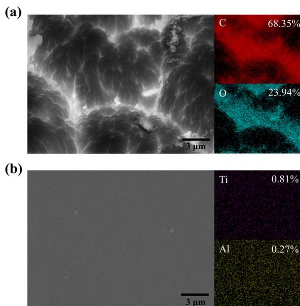
Fig. 7 FESEM images and EDS element mapping of PI and 200 cycles ATO film coated PI after AO erosion: (a) PI surface morphology. (b) ATO@PI surface morphology.
