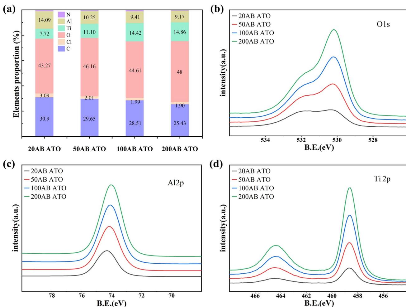
**Fig. 2** The characterization analysis of PI after different ALD cycles. (a) Surface atomic proportions from the XPS spectra analysis. (b) The high-resolution spectra of O 1s. (c) The high-resolution spectra of Al 2p. (d) The high-resolution spectra of Ti 2p.
