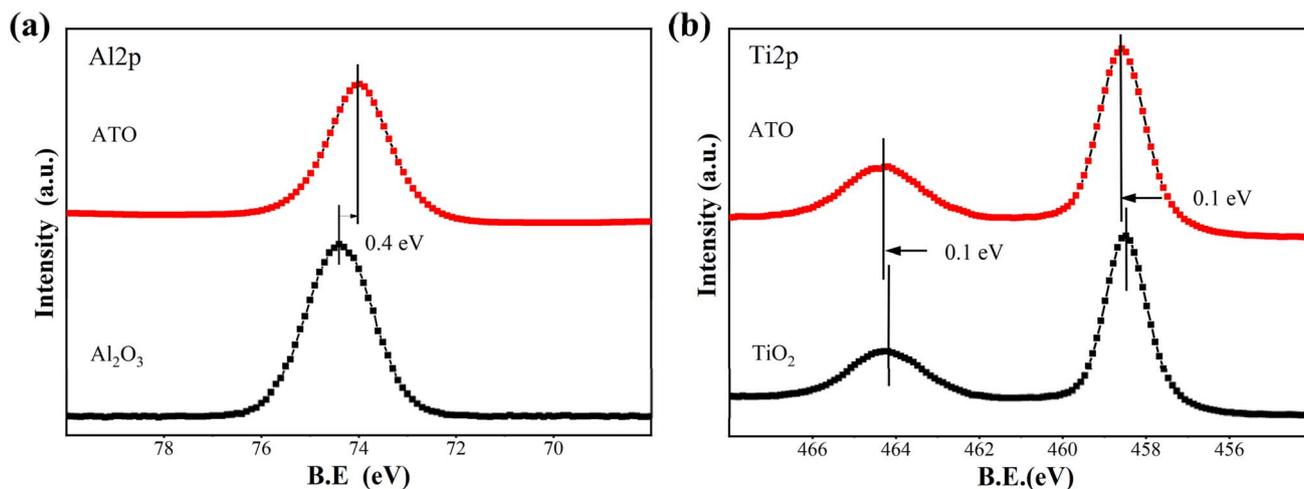
Fig. 5 High-resolution XPS spectra of single  $\text{Al}_2\text{O}_3$ ,  $\text{TiO}_2$  and ATO films on the activated-PI surface after 200 ALD cycles. (a) Al 2p, (b) Ti 2p.
