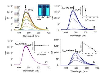
Fig. 6 Photophysical properties of 2 (20  $\mu$ M, MeCN). (Panel A) is the metal screen at  $\lambda_{ex}$  280 nm with 5.0 equivalents of the indicated metal. (Panels B and C) are titration studies for Fe<sup>3+</sup> and Fe<sup>2+</sup> in MeCN, respectively. (Panel D) is the Fe<sup>3+</sup> titration in 7:3 MeCN: H<sub>2</sub>O; cps is counts per second. Cuvette images were taken under the irradiation of a 100 W  $\lambda_{ex}$  365 nm lamp.
