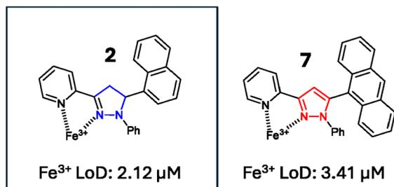
Fig. 16 Proposed 1 : 1 binding mechanism of **2** and **7** with  $\text{Fe}^{3+}$  with the calculated limit of detection for  $\text{Fe}^{3+}$  in 7 : 3 MeCN :  $\text{H}_2\text{O}$  solution. Pyrazoline **2** was selected as the lead compound from this study.
