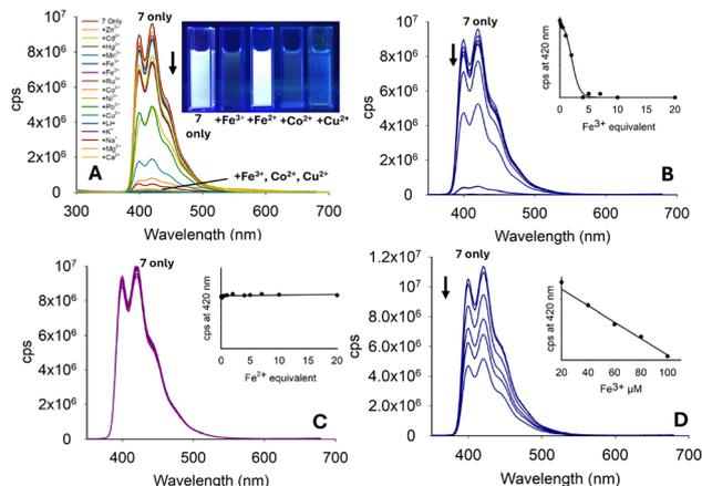
Fig. 10 Photophysical properties of 7 (20  $\mu$ M, MeCN). (Panel A) Metal screen at  $\lambda_{ex}$  280 nm with 5.0 equivalents of the indicated metal. (Panels B and C) Titration studies for Fe<sup>3+</sup> and Fe<sup>2+</sup> in MeCN, respectively. (Panel D) Fe<sup>3+</sup> titration in 7:3 MeCN:H<sub>2</sub>O; cps is counts per second. Cuvette images were taken under the irradiation of a 100 W  $\lambda_{ex}$  365 nm lamp.
