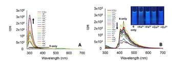
Fig. 9 (Panel A) Metal screen for 5 (20  $\mu$ M, MeCN) at  $\lambda_{ex}$  280 nm with 5.0 equivalents of the indicated metal. (Panel B) Metal screen for 6 at  $\lambda_{ex}$  250 nm in MeCN; cps is counts per second. Cuvette images were taken under the irradiation of a 100 W  $\lambda_{ex}$  365 nm lamp.
