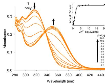
Fig. 2 UV/vis study for 1 (20 μM, MeCN) with 0–20 equivalents of Zn<sup>2+</sup>.
