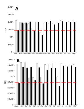
Fig. 12 Competition assays for 2 (Panel A) and 7 (Panel B). The white bar represents the sensor (20  $\mu\text{M},$  MeCN) with 5.0 equivalents of the indicated cation; the black bars is the same with 5.0 equivalents Fe $^{3+}$  after equilibrating for 3 min. 2  $\lambda_{ex}$  280 nm with  $\lambda_{em}$  490 nm; 7  $\lambda_{ex}$  250 nm with  $\lambda_{em}$  420 nm.
