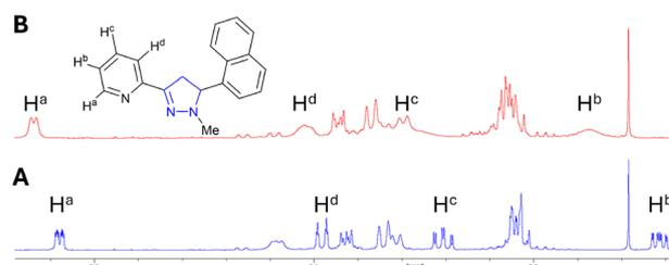
Fig. 3 Partial <sup>1</sup>H NMR spectra: (A) is 1 (20 μM, CDCl<sub>3</sub>) and (B) is 1 + 2.0 equivalents of Zn<sup>2+</sup>.
