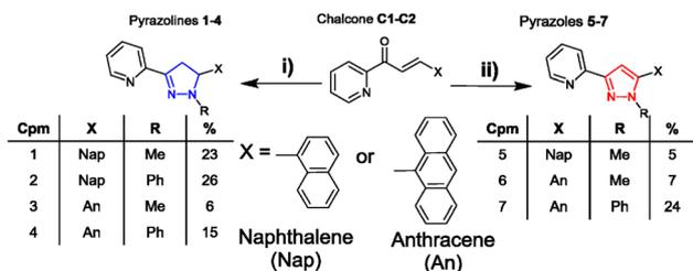
Scheme 2 Synthesis of seven novel sensors from shared chalcone precursors: (i) 2.0 equivalent hydrazine (H<sub>2</sub>NNHMe or H<sub>2</sub>NNHPh), MeOH, 60 °C, and 24 h (ref. 15) (ii) is the same as (i) + 1.0 equivalent CuCl<sub>2</sub>.<sup>16</sup>
