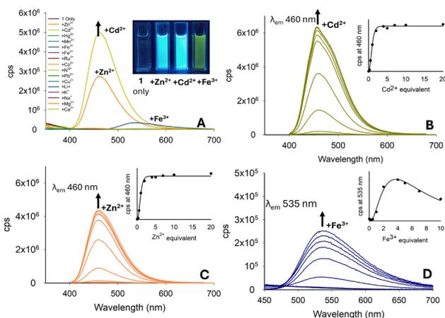
Fig. 5 Photophysical properties of **1** ( $20\ \mu\text{M}$ ,  $\text{MeCN}$ ). (Panel A) Metal screen at  $\lambda_{\text{ex}}\ 280\ \text{nm}$  with 5.0 equivalents of the indicated metal. (Panels B–D) Titration studies for  $\text{Cd}^{2+}$ ,  $\text{Zn}^{2+}$  and  $\text{Fe}^{3+}$ , respectively; cps is counts per second. Cuvette images were taken under the irradiation of a  $100\ \text{W}\ \lambda_{\text{ex}}\ 365\ \text{nm}$  lamp.
