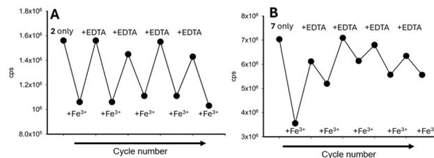
Fig. 15 Repeatability study of the addition of 5.0 equivalents of  $\text{Fe}^{3+}$ , followed by 5.0 equivalents of EDTA, repeated for 5 cycles in a 7 : 3 MeCN :  $\text{H}_2\text{O}$  solution. (Panel A) is 2  $\lambda_{\text{ex}}$  280 nm and (Panel B) is 7  $\lambda_{\text{ex}}$  250 nm; cps is counts per second.
