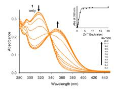
Fig. 2 UV/vis study for 1 (20  $\mu\text{M},$  MeCN) with 0–20 equivalents of  $\text{Zn}^{2+}.$
