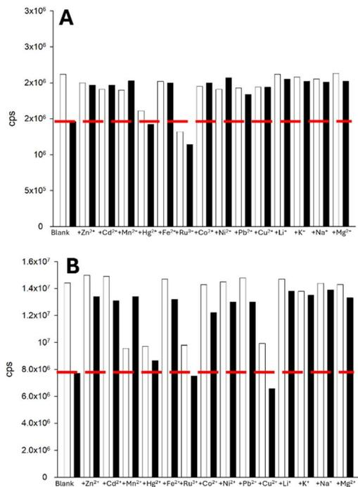
Fig. 12 Competition assays for 2 (Panel A) and 7 (Panel B). The white bar represents the sensor (20  $\mu\text{M}$ , MeCN) with 5.0 equivalents of the indicated cation; the black bars is the same with 5.0 equivalents  $\text{Fe}^{3+}$  after equilibrating for 3 min. 2  $\lambda_{\text{ex}}$  280 nm with  $\lambda_{\text{em}}$  490 nm; 7  $\lambda_{\text{ex}}$  250 nm with  $\lambda_{\text{em}}$  420 nm.
