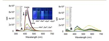
Fig. 7 Photophysical properties of 3 (20  $\mu$ M, MeCN) (Panel A) and 4 (Panel B) metal screen at  $\lambda_{ex}$  250 nm with 5.0 equivalents of the indicated metal; cps is counts per second. Cuvette images were taken under the irradiation of a 100 W  $\lambda_{ex}$  365 nm lamp.
