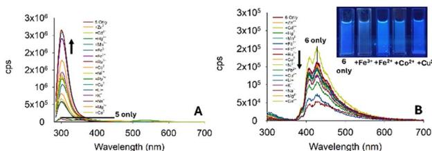
Fig. 9 (Panel A) Metal screen for 5 (20  $\mu$ M, MeCN) at  $\lambda_{ex}$  280 nm with 5.0 equivalents of the indicated metal. (Panel B) Metal screen for 6 at  $\lambda_{ex}$  250 nm in MeCN; cps is counts per second. Cuvette images were taken under the irradiation of a 100 W  $\lambda_{ex}$  365 nm lamp.
