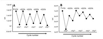
Fig. 15 Repeatability study of the addition of 5.0 equivalents of Fe³+, followed by 5.0 equivalents of EDTA, repeated for 5 cycles in a 7:3 MeCN: H<sub>2</sub>O solution. (Panel A) is 2  $\lambda_{\rm ex}$  280 nm and (Panel B) is 7  $\lambda_{\rm ex}$  250 nm; cps is counts per second.
