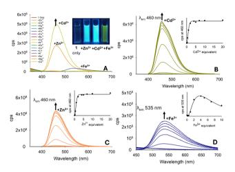
Fig. 5 Photophysical properties of 1 (20  $\mu$ M, MeCN). (Panel A) Metal screen at  $\lambda_{ex}$  280 nm with 5.0 equivalents of the indicated metal. (Panels B–D) Titration studies for Cd²+, Zn²+ and Fe³+, respectively; cps is counts per second. Cuvette images were taken under the irradiation of a 100 W  $\lambda_{ex}$  365 nm lamp.
