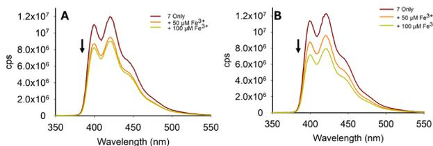
Fig. 13  $\text{Fe}^{3+}$ -triggered "turn-off" response for 7 in tap water (Panel A).  $\text{Fe}^{3+}$ -triggered "turn-off" response for 7 in mineral water (Panel B),  $\lambda_{\text{ex}}$  250 nm. Solvent was 7 : 3 MeCN :  $\text{H}_2\text{O}$ ; cps is counts per second.
