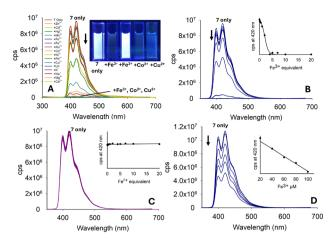
Fig. 10 Photophysical properties of 7 (20  $\mu$ M, MeCN). (Panel A) Metal screen at  $\lambda_{ex}$  280 nm with 5.0 equivalents of the indicated metal. (Panels B and C) Titration studies for Fe<sup>3+</sup> and Fe<sup>2+</sup> in MeCN, respectively. (Panel D) Fe<sup>3+</sup> titration in 7:3 MeCN: H<sub>2</sub>O; cps is counts per second. Cuvette images were taken under the irradiation of a 100 W  $\lambda_{ex}$  365 nm lamp.
