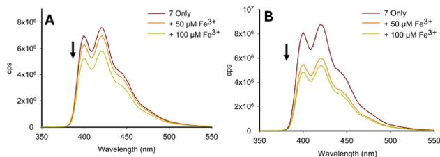
Fig. 14  $\text{Fe}^{3+}$ -triggered "turn-off" response for 7 in pond water (Panel A).  $\text{Fe}^{3+}$ -triggered "turn-off" response for 7 in river water (Panel B),  $\lambda_{\text{ex}}$  250 nm. Solvent composition was 7 : 3 MeCN :  $\text{H}_2\text{O}$ ; cps is counts per second.
