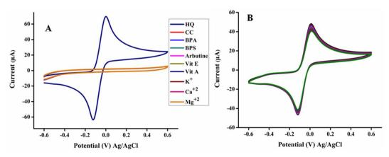
Fig. 7 (A) Anti-interference behavior of poly (quinine-co-itaconic acid)@rGO and (B) stability of poly (quinine-co-itaconic acid)@rGO.
