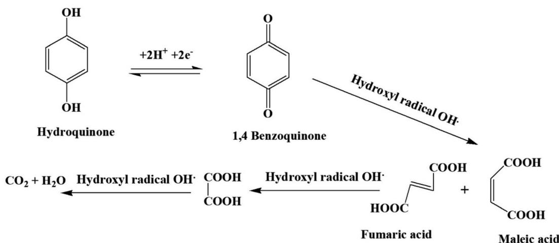
Fig. 13 Schematic representation of photocatalytic degradation of HQ.
