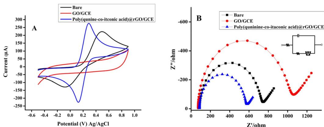
Fig. 5 (A) CV, (B) EIS response of bare/GCE, graphene oxide/GCE and poly (quinine-co-itaconic acid)@rGO/GCE.
