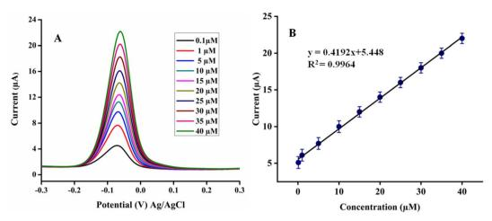
(A) Calibration plot of HQ (B) plot of linear regression equation.
