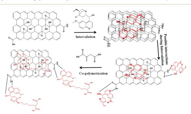
Fig. 1 Schematic diagram for the synthesis of poly (quinine-co-itaconic acid)@rGO.
