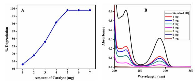
Fig. 10 (A) % Degradation of HQ at different amounts of catalyst and (B) UV-vis spectra of photocatalytic degradation of HQ at different amounts of catalyst.
