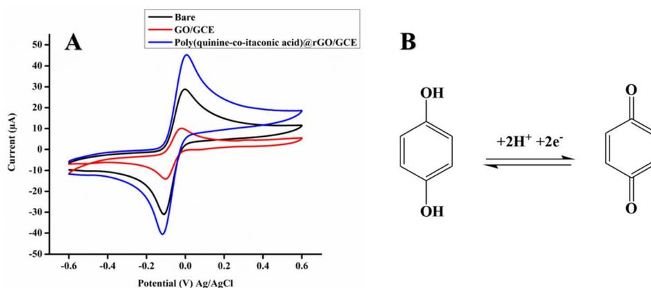
Fig. 6 (A) CV redox response of bare, GO/GCE and poly (quinine-*co*-itaconic acid)@rGO/GCE in 10  $\mu$ M HQ at scan rate 50 mV s<sup>-1</sup> in borate buffer of pH 8 and (B) possible mechanism for HQ at poly (quinine-*co*-itaconic acid)@rGO/GCE.
