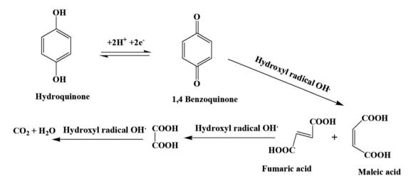
Fig. 13 Schematic representation of photocatalytic degradation of HQ
