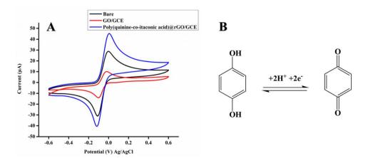
Fig. 6 (A) CV redox response of bare, GO/GCE and poly (quinine-co-itaconic acid)@rGO/GCE in 10  $\mu$ M HQ at scan rate 50 mV s<sup>-1</sup> in borate buffer of pH 8 and (B) possible mechanism for HQ at poly (quinine-co-itaconic acid)@rGO/GCE.
