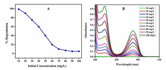
Fig. 11 (A) % Degradation at different concentration of HQ and (B) UV-vis spectra of photocatalytic degradation of HQ at different concentration.
