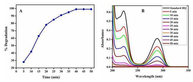
Fig. 9 (A) % Degradation of HQ at different time intervals and (B) UV-vis spectra of photocatalytic degradation of HQ at different time intervals.
