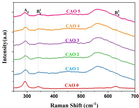
Fig. 6 Raman spectra of spray-deposited CAO films.
