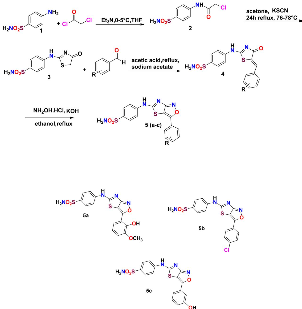
Scheme 1 Schematic of the four-step synthesis of sulfonamide derivatives and their structures (YM-1 (5a), YM-2 (5b), YM-3 (5c)).
