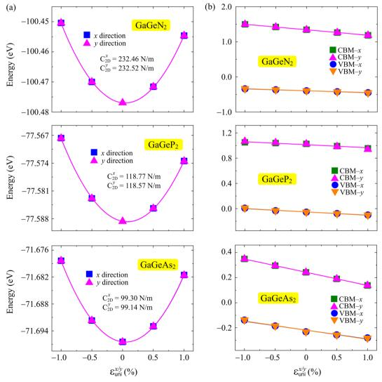
Fig. 7 The total energy (a) and band edges (b) dependence on applied strains in the x/y directions of GaGeX<sub>2</sub> systems. The fitted curves are indicated by the solid lines.
