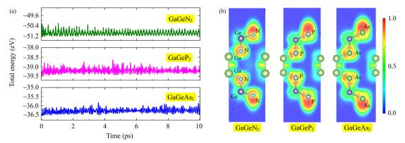
Fig. 2 (a) The total energy-simulation time dependences at 300 K by AIMD calculations and (b) electron localization function (ELF) of GaGeX<sub>2</sub> structures. The high–low charge densities are indicated by the red-blue regions.
