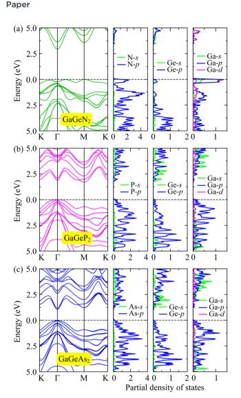
Fig. 5 Calculated HSE06 + SOC band structures and corresponding partial density of states of GaGeN2 (a), GaGeP2 (b), and GaGeAs2 (c) monolayers.
