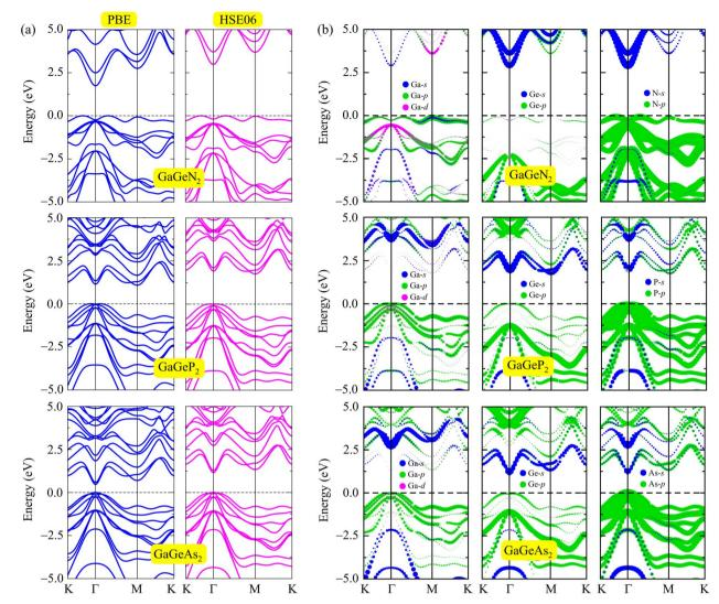
Fig. 4 (a) Electronic band structures at PBE/HSE06 levels and (b) weighted band structures of GaGeN<sub>2</sub>, GaGeP<sub>2</sub>, and GaGeAs<sub>2</sub> monolayers with the Fermi level indicated by the dashed horizontal line at zero.
