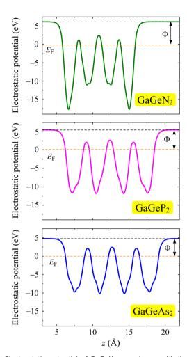
Electrostatic potential of GaGeX<sub>2</sub> monolayers with the dipole correction. The dashed orange lines indicate the Fermi level.
