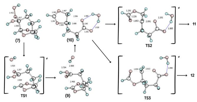
Scheme 4 Geometries of the species involved in the reaction, computed at IEFPCM( $H_2O$ )/M06-2X/6-311++G(d,p) level. Selected geometric parameters are shown, when appropriate.
