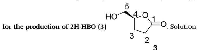
A: Cyrene™ (4.61 mL, 45 mmol) in 2.84 mL of H<sub>2</sub>O (6.04 M), solution B: H<sub>2</sub>O<sub>2</sub> 30% (v/v) (5.57 mL, 54 mmol, 1.2 eq) in 0.715 mL of H<sub>2</sub>O (8 M). The solutions were pumped with a Syrris® syringe pump, mixed in a T connector, and passed through
