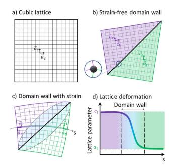
Fig. 6 Schematic representations of the cubic lattice (a) in the HT phase, and two tetragonal domains in the LT phase (b) with the tetragonal axis  $c_t$  horizontal (purple) or vertical (green) for a strain-free domain wall. The inset shows the distortion of the metallic sites on the wall. (c) Domain wall with strained region represented by the blue shaded elliptical area. (d) Evolution of the lattice parameter through the domain wall.
