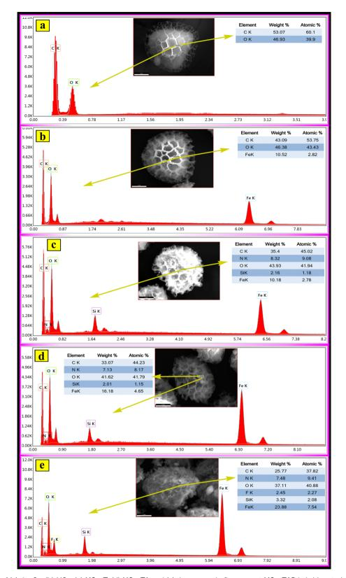
Fig. 6 EDX results of (a) the Sp, (b) MSp, (c) MSp-T, (d) MSp-TA and (e) the magnetic fluorescent MSp-TAB hybrid material.
