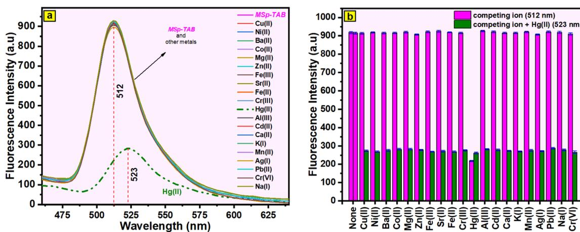
Fig. 8 (a) Fluorescence emission spectra (460–650 nm) of the magnetic fluorescent MSP-TAB hybrid material ( $0.15 \text{ g L}^{-1}$  in ethyl alcohol/water (3/7)) after the addition of different cations. (b) Emission intensity changes at 512 nm and 523 nm of the magnetic fluorescent MSP-TAB hybrid material ( $0.15 \text{ g L}^{-1}$  in ethyl alcohol/water (3/7)) in the presence of other metals with/without Hg(II). (Error analysis has been marked with error bars).
