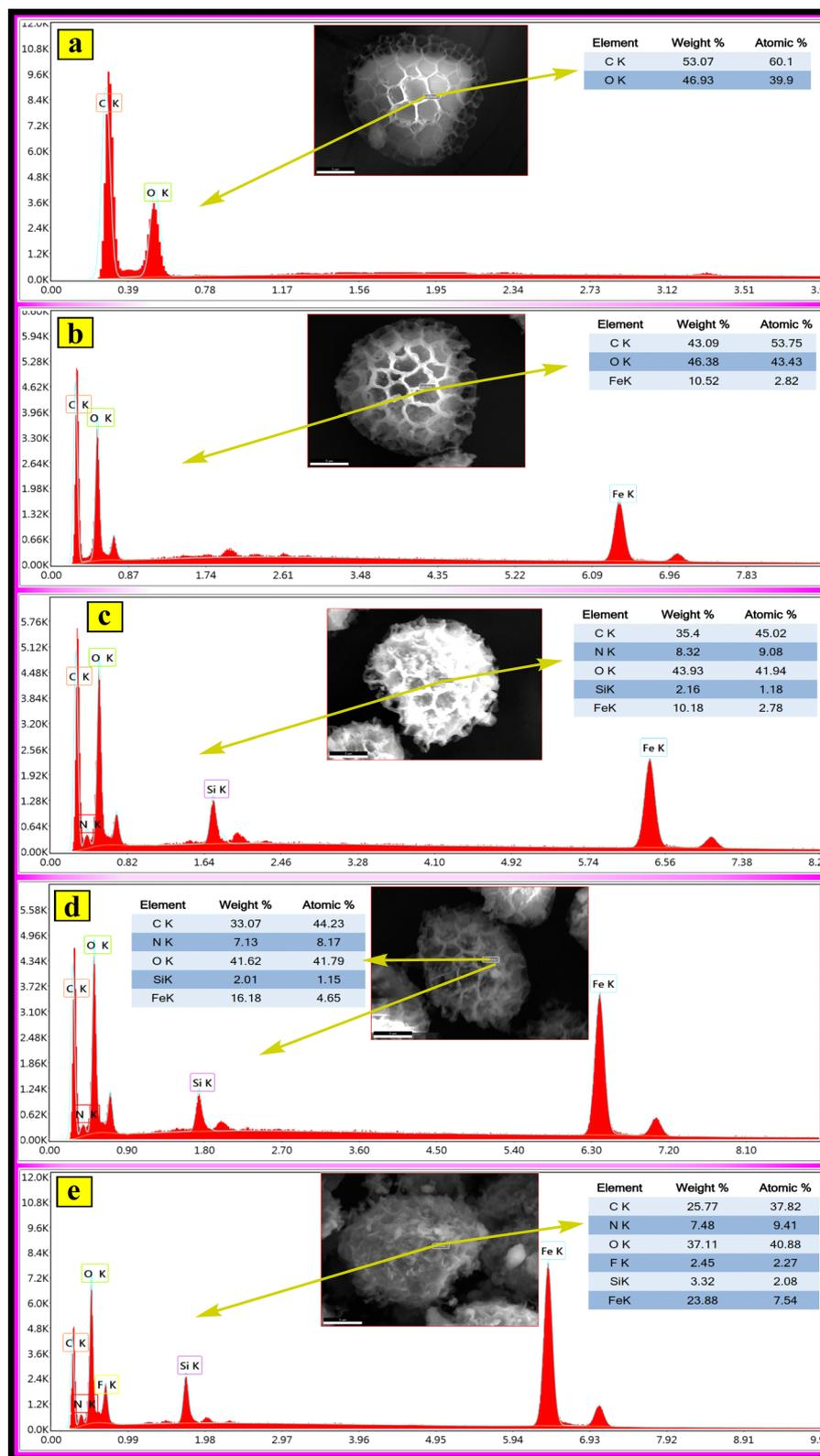
Fig. 6 EDX results of (a) the Sp, (b) MSp, (c) MSp-T, (d) MSp-TA and (e) the magnetic fluorescent MSp-TAB hybrid material.
