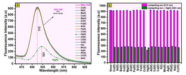
Fig. 8 (a) Fluorescence emission spectra (460–650 nm) of the magnetic fluorescent MSp-TAB hybrid material (0.15 g  $L^{-1}$  in ethyl alcohol/water (3/7)) after the addition of different cations. (b) Emission intensity changes at 512 nm and 523 nm of the magnetic fluorescent MSp-TAB hybrid material (0.15 g  $L^{-1}$  in ethyl alcohol/water (3/7)) in the presence of other metals with/without Hg(II). (Error analysis has been marked with error bars).
