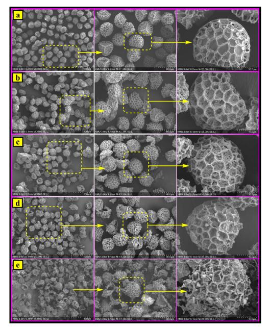
Fig. 5 SEM images for (a) the Sp, (b) MSp, (c) MSp-T, (d) MSp-TA and (e) the magnetic fluorescent MSp-TAB hybrid material.
