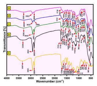
Fig. 2 The FT-IR spectra of (a) the Sp, (b) MSp, (c) MSp-T, (d) MSp-TA and (e) the magnetic fluorescent MSp-TAB hybrid material.
