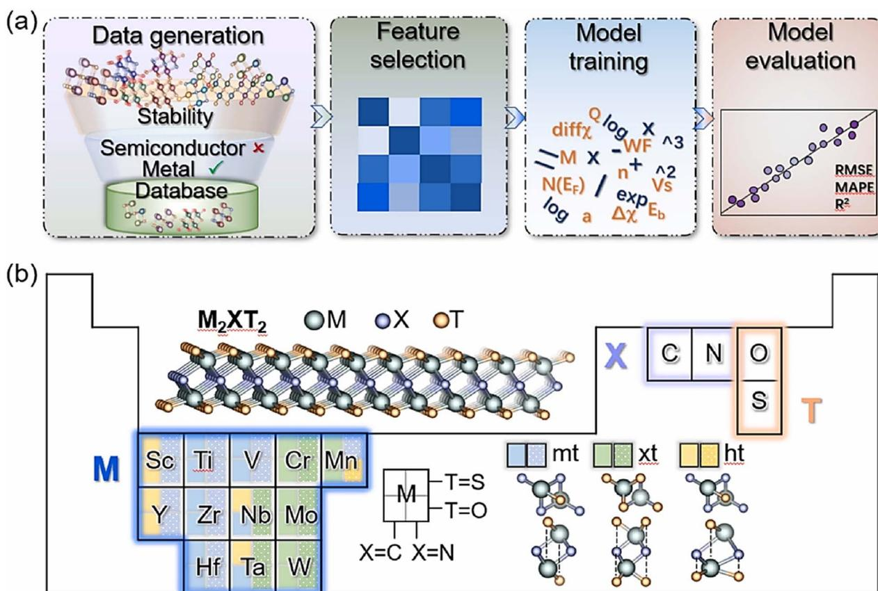
Fig. 6 (a) The process flow of ML is illustrated in the workflow diagram. (b) The distribution of elements and structures within  $\text{M}_2\text{XT}_2$  (T = bare, O, S). Reproduced with permission from ref. 11. Copyright 2023 Elsevier.
