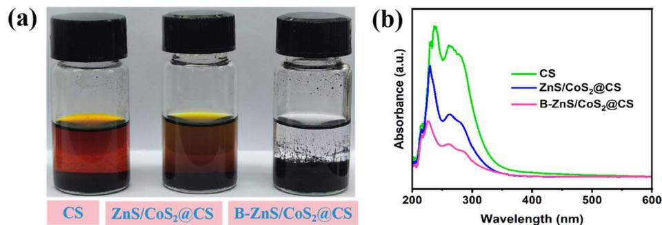
Fig. 8 (a) Digital photographs and (b) UV-vis spectra of different catalysts after soaking in  $\text{Li}_2\text{S}_6$ .
