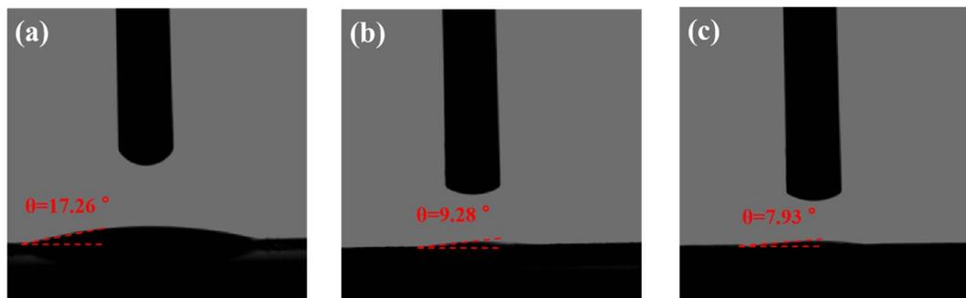
Fig. 11 The electrolyte contact angles of different separators: (a) CS, (b) ZnS/CoS<sub>2</sub>@CS, and (c) B–ZnS/CoS<sub>2</sub>@CS.
