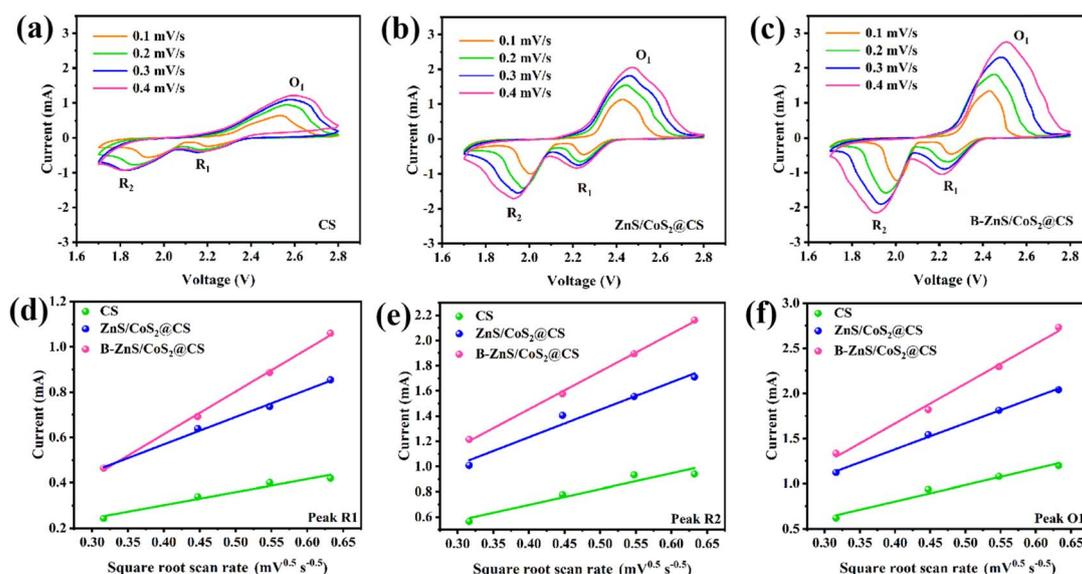
Fig. 13 (a) CV curves of LSBs assembled by CS, (b) ZnS/CoS<sub>2</sub>@CS and (c) B-ZnS/CoS<sub>2</sub>@CS catalyst-modified separators at different scan rates, and the relationship between the peak current and square root of the scan rate: (d) R1 peak, (e) R2 peak, and (f) O1 peak.
