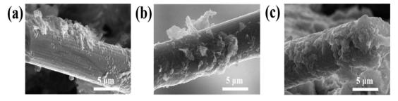
Fig. 17 SEM images of the Li<sub>2</sub>S deposition on different catalyst electrodes: (a) CS; (b) ZnS/CoS<sub>2</sub>@CS and (c) B-ZnS/CoS<sub>2</sub>@CS
