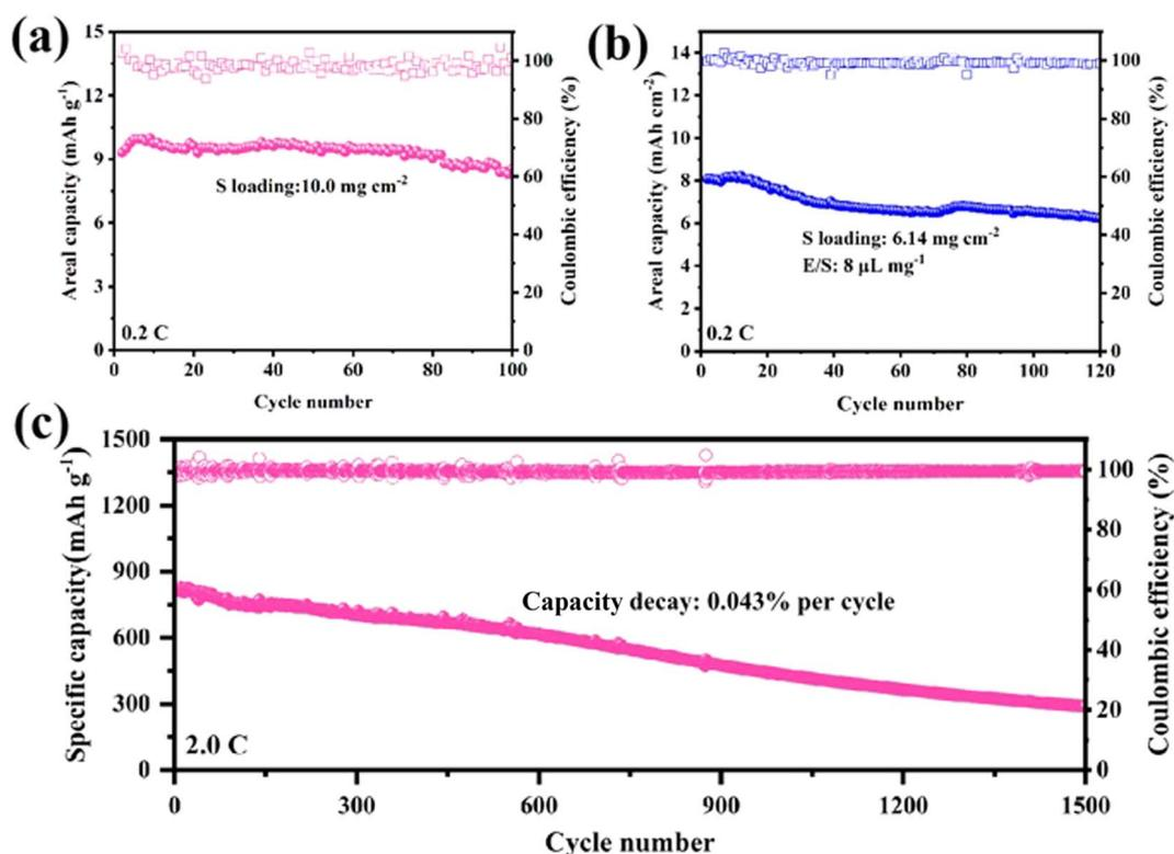
Fig. 22 The cycle performance of LSBs assembled with the B-ZnS/CoS<sub>2</sub>@CS separator: (a) 10.0 mg cm<sup>-2</sup> high sulfur loading cycle performance, (b) 6.14 mg cm<sup>-2</sup> high sulfur loading cycle performance at low E/S ratio, and (c) 2.0C long-cycle performance.
