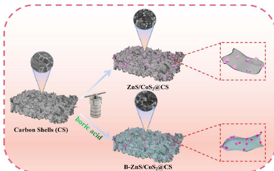
Fig. 1 The schematic diagram of the preparation process of B-ZnS/CoS<sub>2</sub>@CS.
