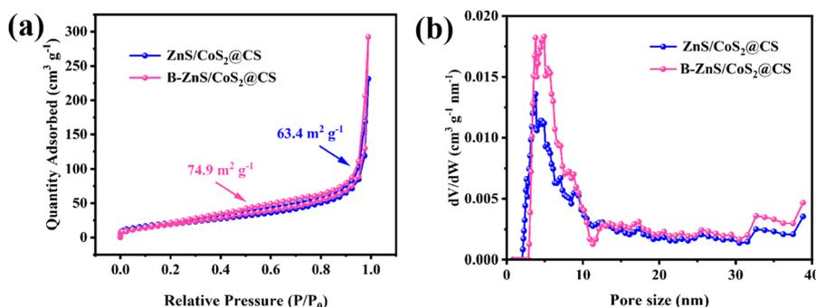
Fig. 6 Pore structure of ZnS/CoS<sub>2</sub>@CS and B-ZnS/CoS<sub>2</sub>@CS: (a) N<sub>2</sub> adsorption–desorption curve and (b) pore size distribution.
