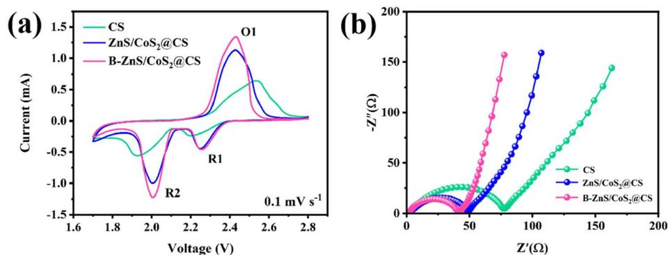
Fig. 12 (a) CV curves and (b) AC impedance spectra of LSBs assembled by the CS, ZnS/CoS<sub>2</sub>@CS and B-ZnS/CoS<sub>2</sub>@CS catalyst-modified separators.
