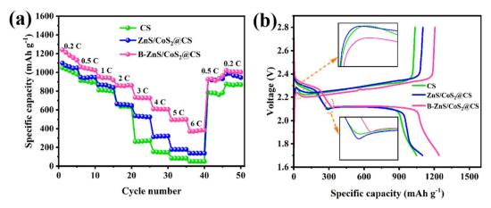
Rate performance of batteries assembled with different separators: (a) rate performance and (b) charge/discharge curve of the 0.2C first cycle.
