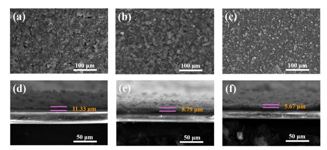
Fig. 10 Top SEM images of (a–c) CS, ZnS/CoS<sub>2</sub>@CS and B–ZnS/CoS<sub>2</sub>@CS-modified separators. Cross-sectional SEM images of (d–f) CS, ZnS/CoS<sub>2</sub>@CS and B–ZnS/CoS<sub>2</sub>@CS-modified separators.
