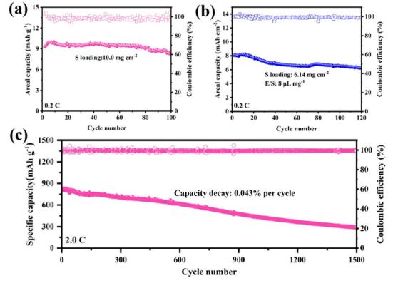
Fig. 22 The cycle performance of LSBs assembled with the  $B-ZnS/CoS_2@CS$  separator: (a) 10.0 mg cm<sup>-2</sup> high sulfur loading cycle performance, (b) 6.14 mg cm<sup>-2</sup> high sulfur loading cycle performance at low E/S ratio, and (c) 2.0C long-cycle performance.
