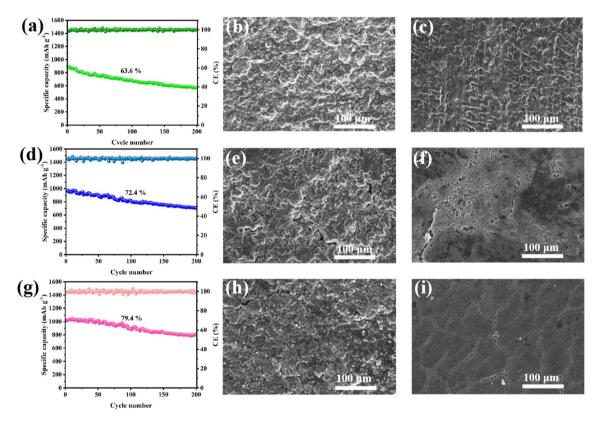
Fig. 20 0.5C cycle performance and SEM images of separators and lithium plates after cycling: (a) CS, (d) ZnS/CoS<sub>2</sub>@CS, and (g) B-ZnS/ CoS<sub>2</sub>@CS, corresponding to (b, e and h) separators and (c, f and i) lithium plates after cycling.
