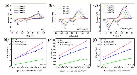
Fig. 13 (a) CV curves of LSBs assembled by CS, (b)  $ZnS/CoS_2@CS$  and (c)  $B-ZnS/CoS_2@CS$  catalyst-modified separators at different scan rates, and the relationship between the peak current and square root of the scan rate: (d) R1 peak, (e) R2 peak, and (f) O1 peak.
