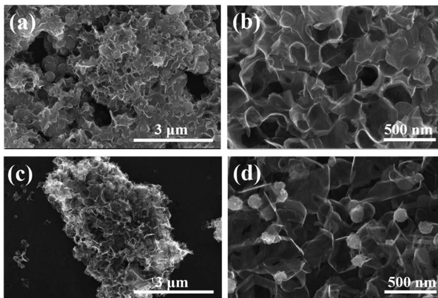
Fig. 3 SEM images of the catalytic materials: (a and b) ZnS/CoS<sub>2</sub>@CS and (c and d) B-ZnS/CoS<sub>2</sub>@CS.
