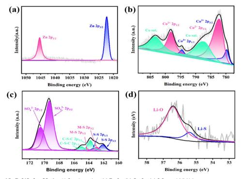
XPS spectra of B-ZnS/CoS<sub>2</sub>@CS after Li<sub>2</sub>S<sub>6</sub> adsorption: (a) Zn 2p, (b) Co 2p, (c) S 2p and (d) Li 1s.
