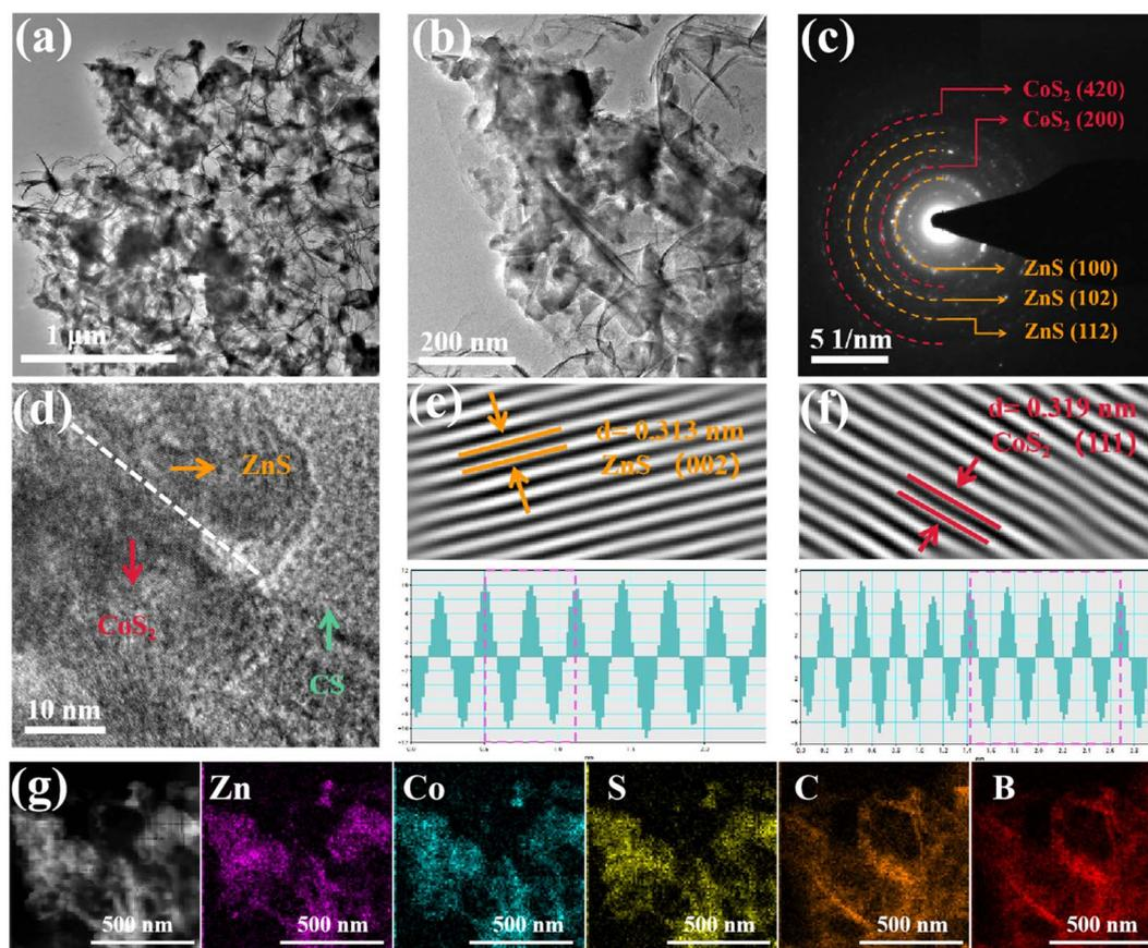
Fig. 4 (a and b) TEM image, (c) SAED pattern, (d–f) HRTEM image of B-ZnS/CoS<sub>2</sub>@CS, and (g) EDX mapping results.
