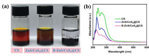
(a) Digital photographs and (b) UV-vis spectra of different catalysts after soaking in Li<sub>2</sub>S<sub>6</sub>.
