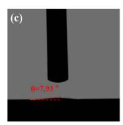
Fig. 11 The electrolyte contact angles of different separators: (a) CS, (b) ZnS/CoS<sub>2</sub>@CS, and (c) B-ZnS/CoS<sub>2</sub>@CS.
