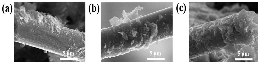
Fig. 17 SEM images of the Li<sub>2</sub>S deposition on different catalyst electrodes: (a) CS; (b) ZnS/CoS<sub>2</sub>@CS and (c) B-ZnS/CoS<sub>2</sub>@CS.
