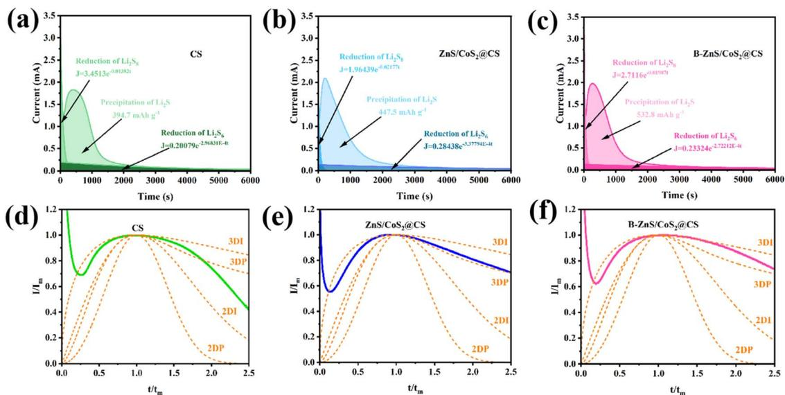
Fig. 16 Potentiostatic discharge curves of the Li<sub>2</sub>S<sub>8</sub> electrolyte at 2.05 V on the (a) CS, (b) ZnS/CoS<sub>2</sub>@CS, and (c) B-ZnS/CoS<sub>2</sub>@CS cathodes, and dimensionless  $i-t$  transient fitting results of the Li<sub>2</sub>S nucleation process on the (d) CS, (e) ZnS/CoS<sub>2</sub>@CS and (f) B-ZnS/CoS<sub>2</sub>@CS catalysts.
