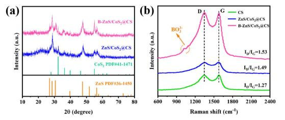
Fig. 5 Physical properties of different catalysts: (a) XRD and (b) Raman results.
