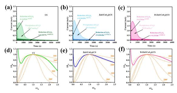
Fig. 16 Potentiostatic discharge curves of the Li<sub>2</sub>S<sub>8</sub> electrolyte at 2.05 V on the (a) CS, (b) ZnS/CoS<sub>2</sub>@CS, and (c) B-ZnS/CoS<sub>2</sub>@CS cathodes, and dimensionless i-t transient fitting results of the Li<sub>2</sub>S nucleation process on the (d) CS, (e) ZnS/CoS<sub>2</sub>@CS and (f) B-ZnS/CoS<sub>2</sub>@CS catalysts.
