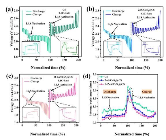
Fig. 18 GITT curves of (a) CS, (b) ZnS/CoS<sub>2</sub>@CS, (c)  $B-ZnS/CoS_2$ @CS batteries, and (d) the internal resistance of different batteries based on the normalized discharge/charge time.
