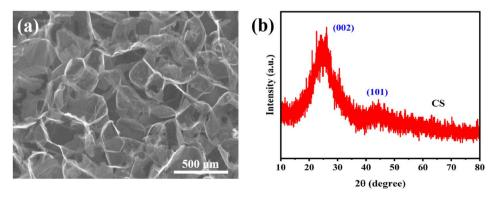
Fig. 2 The morphology and phase structure of CS: (a) SEM and (b) XRD result.
