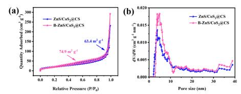
Pore structure of ZnS/CoS<sub>2</sub>@CS and B-ZnS/CoS<sub>2</sub>@CS: (a) N<sub>2</sub> adsorption-desorption curve and (b) pore size distribution.
