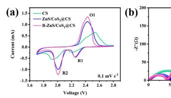
Fig. 12 (a) CV curves and (b) AC impedance spectra of LSBs assembled by the CS,  $ZnS/CoS_2@CS$  and  $B-ZnS/CoS_2@CS$  catalyst-modified separators.
