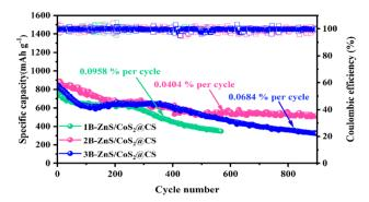
Fig. 21 Comparison of the cycle performance of the B-ZnS/CoS<sub>2</sub>@CS catalyst batteries with different boron doping amounts at 1.0C.
