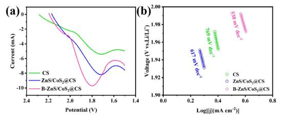
Fig. 15 (a) The LSV curves and (b) the corresponding Tafel curves of CS, ZnS/CoS<sub>2</sub>@CS and B-ZnS/CoS<sub>2</sub>@CS.
