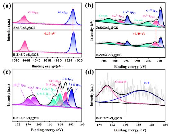
Fig. 7 (a) Zn 2p, (b) Co 2p, (c) S 2p and (d) B 1s XPS spectra of the ZnS/CoS<sub>2</sub>@CS and B-ZnS/CoS<sub>2</sub>@CS catalysts.
