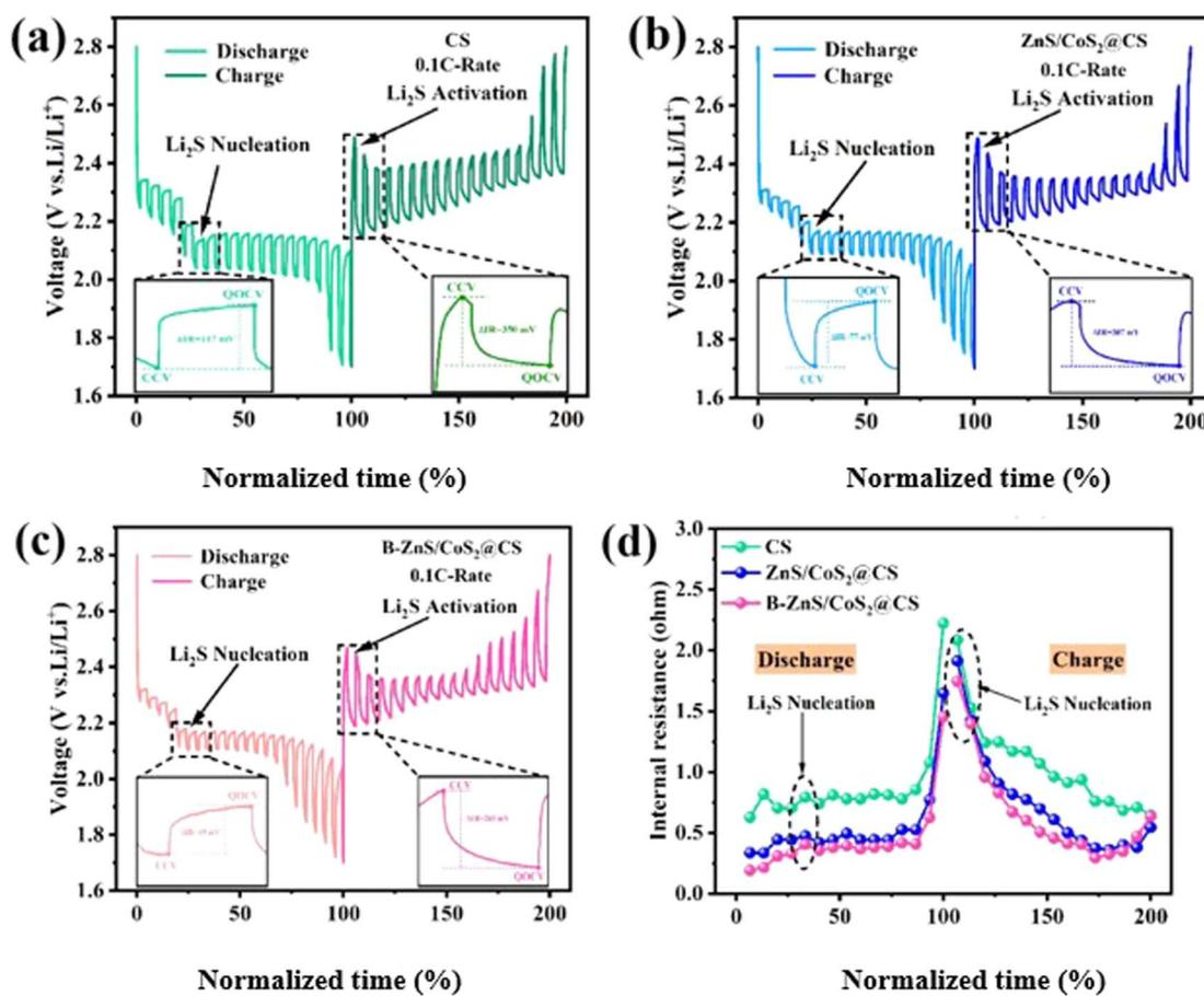
Fig. 18 GITT curves of (a) CS, (b) ZnS/CoS<sub>2</sub>@CS, (c) B-ZnS/CoS<sub>2</sub>@CS batteries, and (d) the internal resistance of different batteries based on the normalized discharge/charge time.
