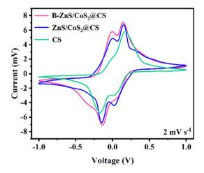
Fig. 14 CV of symmetric cells assembled by CS, ZnS/CoS<sub>2</sub>@CS and B–ZnS/CoS<sub>2</sub>@CS.
