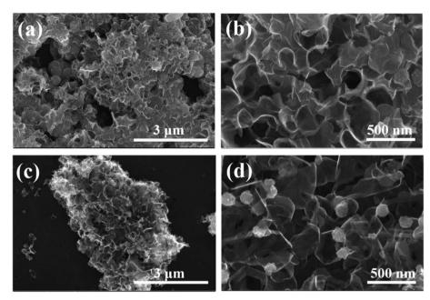
Fig. 3 SEM images of the catalytic materials: (a and b) ZnS/CoS2@CS and (c and d) B-ZnS/CoS2@CS.
