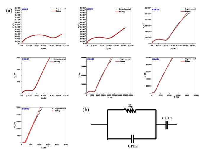
Fig. 5 (a) Nyquist plot for pristine polymer and  $MgCl_2$  salt added electrolyte samples. (b) Model of the equivalent circuit.
