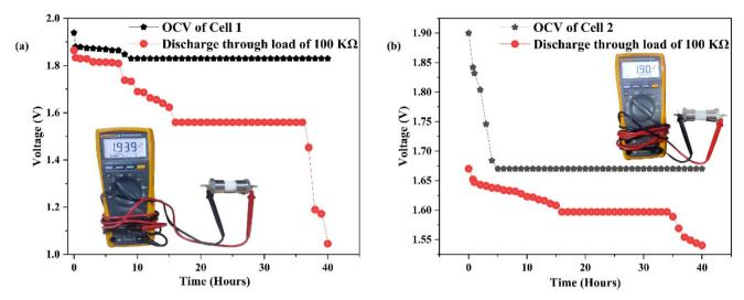
Fig. 14 (a) The open circuit voltage (OCV) of cell 1 (photo of cell 1 shown in the inset). (b) The open circuit voltage (OCV) of cell 2 (photo of cell 2 shown in the inset).
