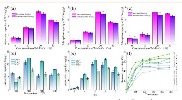
Fig. 3 Effects of MCA1-1, MCA1-2, MCA1-3 and MCA1-4 on adsorption capacity of (a) Pb<sup>2+</sup>, (b) Cu<sup>2+</sup> and (c) Cd<sup>2+</sup>; effect of (d) carbonation temperature, (e) pH and (f) initial concentration on the adsorption capacities of MCA1-3 towards Pb2+, Cu2+ and Cd2+.
