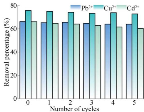
Fig. 7 Removal efficiency of Pb<sup>2+</sup>, Cu<sup>2+</sup> and Cd<sup>2+</sup> by MCA in 5 adsorption-desorption cycles.
