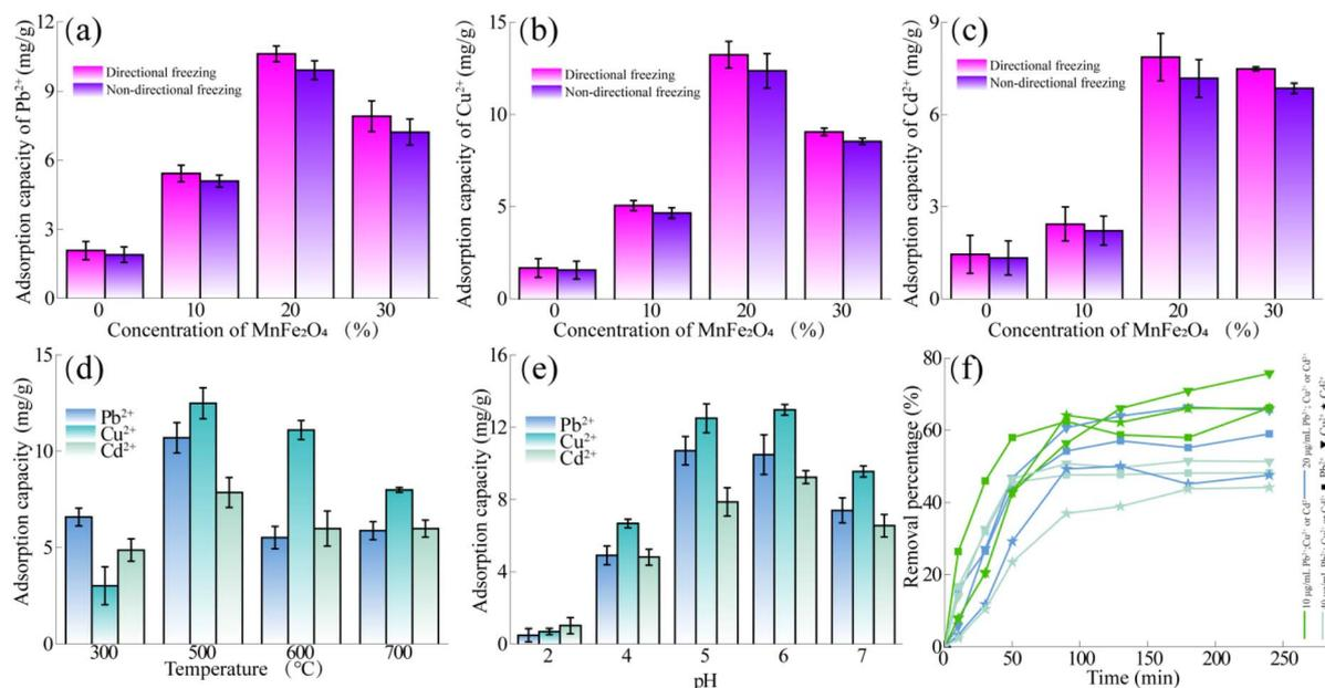
Fig. 3 Effects of MCA1-1, MCA1-2, MCA1-3 and MCA1-4 on adsorption capacity of (a) Pb<sup>2+</sup>, (b) Cu<sup>2+</sup> and (c) Cd<sup>2+</sup>; effect of (d) carbonation temperature, (e) pH and (f) initial concentration on the adsorption capacities of MCA1-3 towards Pb<sup>2+</sup>, Cu<sup>2+</sup> and Cd<sup>2+</sup>.
