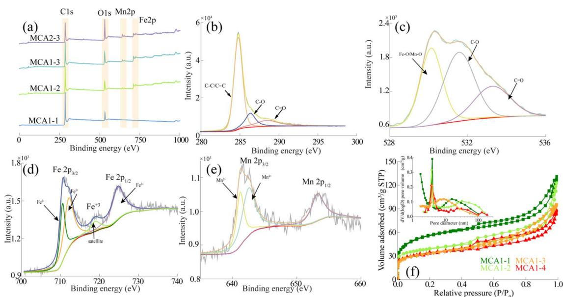
**Fig. 2** (a) XPS spectrum of MCA; high-resolution XPS of MCA1-3: (b) C 1s, (c) O 1s, (d) Fe 2p; (e) Mn 2p; (f)  $\text{N}_2$  adsorption–desorption isothermal curves of MCA, pore size distribution of MCA (inset).
