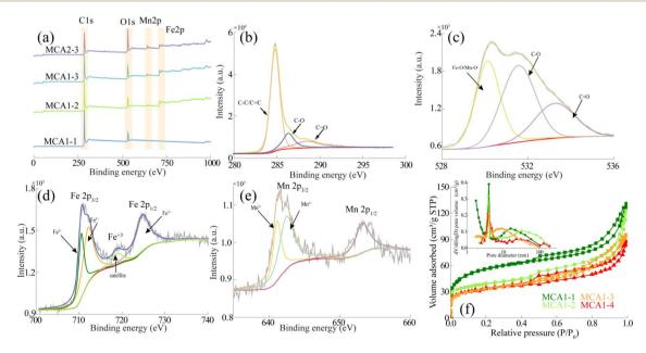
Fig. 2 (a) XPS spectrum of MCA; high-resolution XPS of MCA1-3: (b) C 1s, (c) O 1s, (d) Fe 2p; (e) Mn 2p; (f)  $N_2$  adsorption–desorption isothermal curves of MCA, pore size distribution of MCA (inset).
