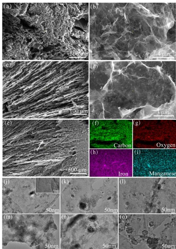
**Fig. 1** (a and b) SEM images of MCA1-1 obtained by non directional freezing at different magnifications; (c–e) SEM images of MCA1-3 obtained by directional freezing at different magnifications; MCA1-3 element mapping ((f) carbon; (g) oxygen; (h) iron; (i) manganese); (j) MCA1-2 (inset: MCA1-1); (k) MCA1-3; (l) MCA1-4; (m) MCA2-1; (n) MCA2-2; (o) MCA2-3.
