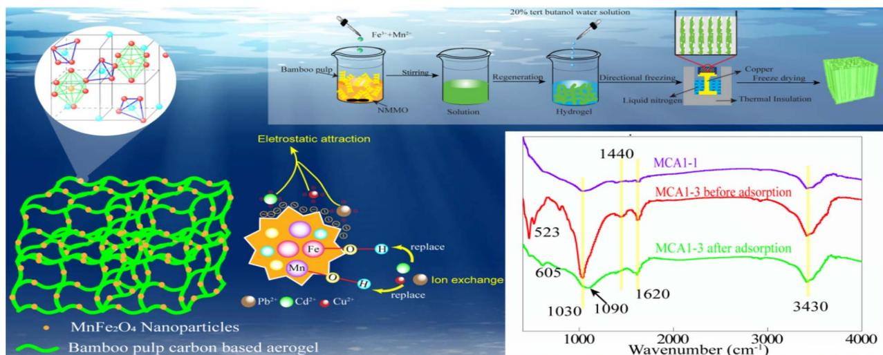
**Fig. 6** FTIR of before and after adsorption and possible mechanism of the adsorption of MCA on Pb<sup>2+</sup>, Cu<sup>2+</sup> and Cd<sup>2+</sup>.
