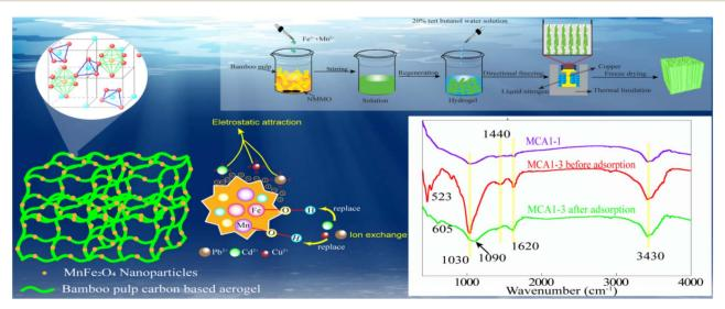
Fig. 6 FTIR of before and after adsorption and possible mechanism of the adsorption of MCA on Pb<sup>2+</sup>, Cu<sup>2+</sup> and Cd<sup>2+</sup>.
