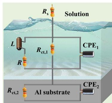
Fig. 4 The equivalent circuit used for fitting the EIS data.
