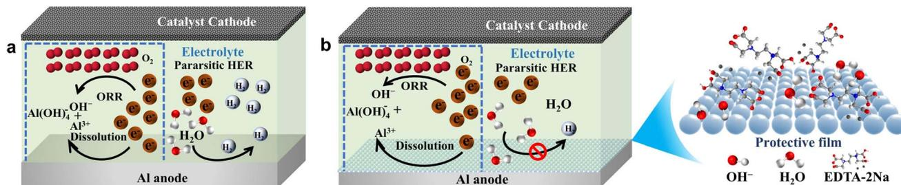
Fig. 9 Proposed mechanism of electrochemical behavior of Al alloy in (a) pristine and (b) inhibited electrolytes.
