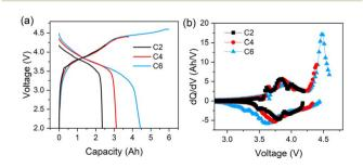
Fig. 1 Formation curves of LLOs-based batteries. (a) Charge and discharge curves (b)  ${\rm d}Q/{\rm d}V$  curves.
