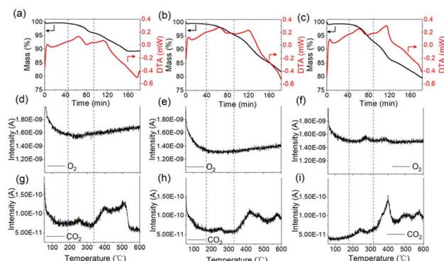
Fig. 4 TG-MS curves of the samples (a, d and g) for CM2; (b, e and h) for CM4; (c, f and i) for CM6.
