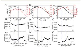
Fig. 4 TG-MS curves of the samples (a, d and g) for CM2; (b, e and h) for CM4; (c, f and i) for CM6).
