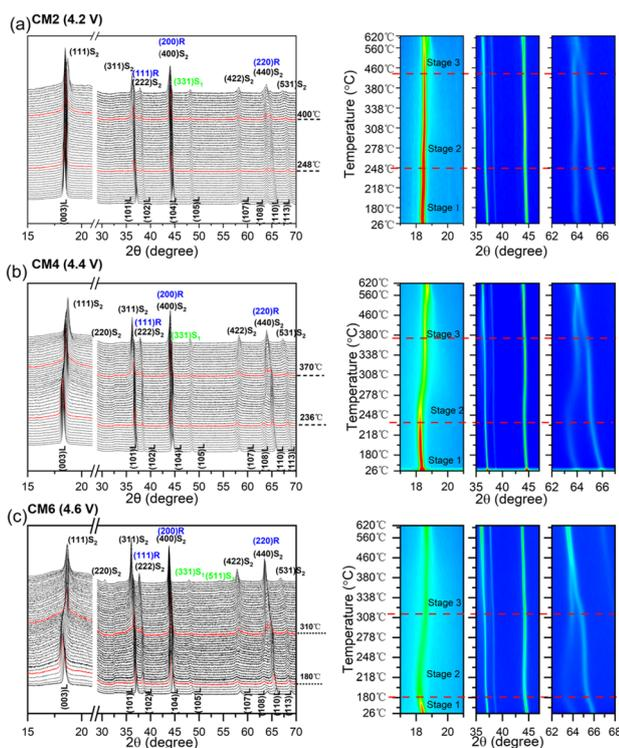
Fig. 5 (a–c) *In situ* HT-XRD patterns and contour images of the cathode materials with different activation voltages (the layered phase, Li<sub>x</sub>Mn<sub>2</sub>O<sub>4</sub>-type spinel phase, Mn<sub>2</sub>NiO<sub>4</sub>-type spinel phase, and rock salts are abbreviated to L, S<sub>1</sub>, S<sub>2</sub> and RS, respectively).
