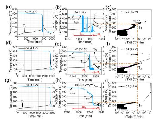
Fig. 2 ARC testing results of all batteries with different upper voltages ((a-c) for 4.2 V, (d-f) for 4.4 V, (q-i) for 4.6 V).
