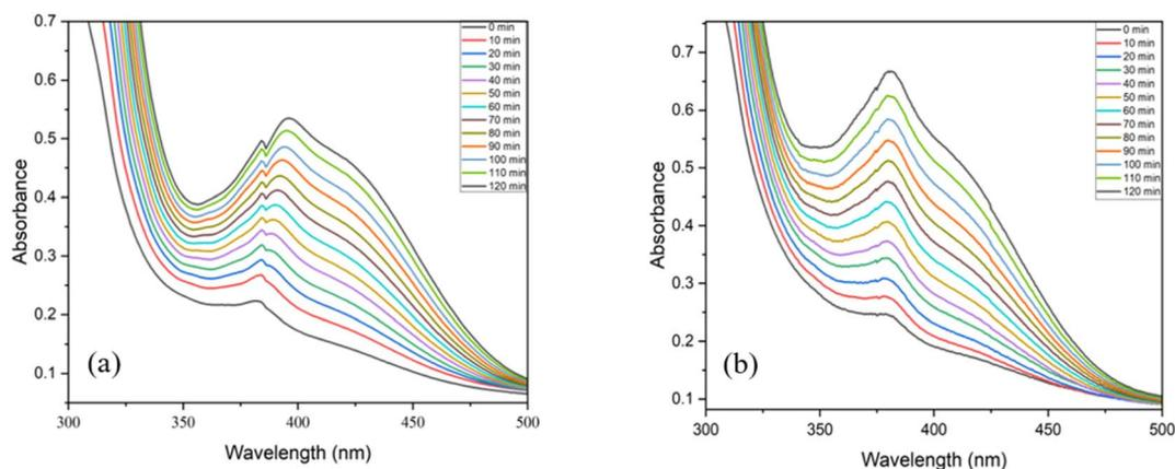
Fig. 8 UV-visible spectra of reaction mixture of C1 recorded at the time interval of 10 min, (a) under ambient conditions, (b) under high O<sub>2</sub> concentration conditions.
