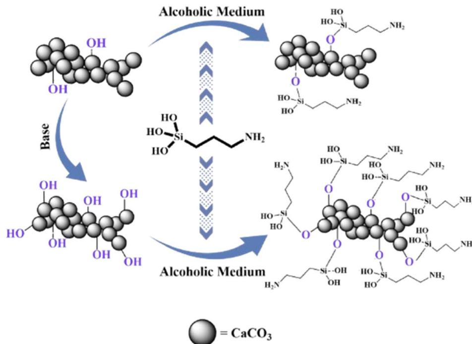
Fig. 2 Surface modification of CC with ATPS.
