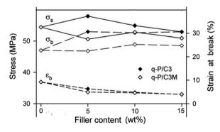
Fig. 4 Tensile strength and strain at break at different wt% values for filler content, adopted from ref. 97 with license 5513130080154.
