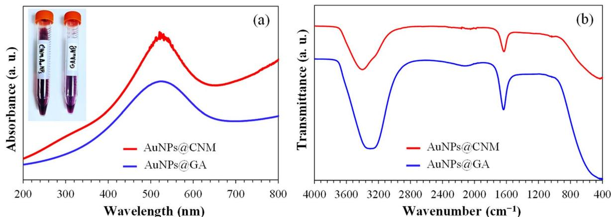
Fig. 5 (a) UV-Vis absorption spectra of the prepared AuNPs@GA and AuNPs@CNM, (b) FTIR spectra of the prepared AuNPs@GA and AuNPs@CNM.
