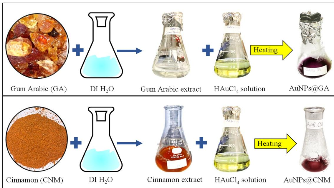
Fig. 1 A schematic diagram showing the synthesis process of AuNPs@GA and AuNPs@CNM using gum Arabic (GA) and cinnamon (CNM).
