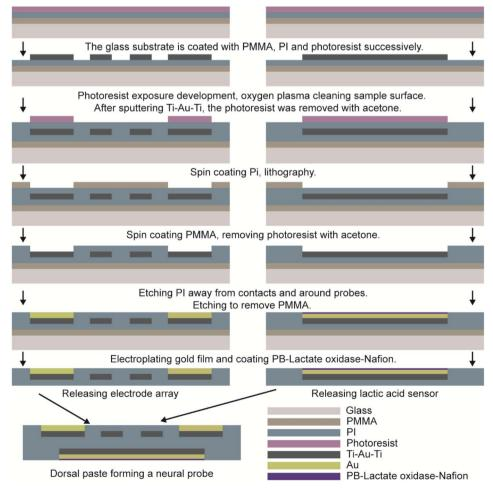
Fig. 2 The complete process flow
