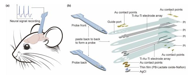
Fig. 1 The flexible multimodal integrated neural probe. (a) Diagram of the probe' functions; (b) diagram of the probe structure.
