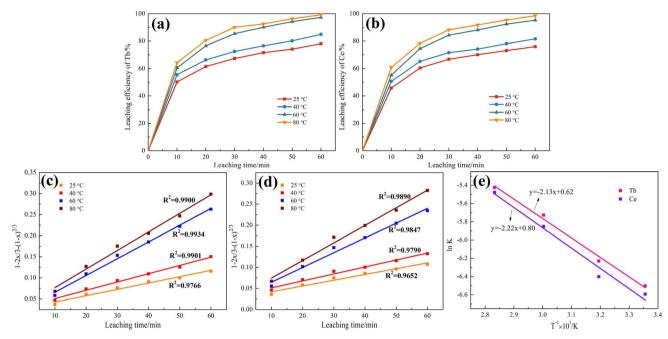
Fig. 3 Leaching efficiencies of (a) Tb and (b) Ce at various temperatures as a function of time, plots of  $1 - 2x/3 - (1 - x)^{2/3} - t$  at various temperatures for (c) Tb and (d) Ce, and (e) plot of  $\ln k - T^{-1}$
