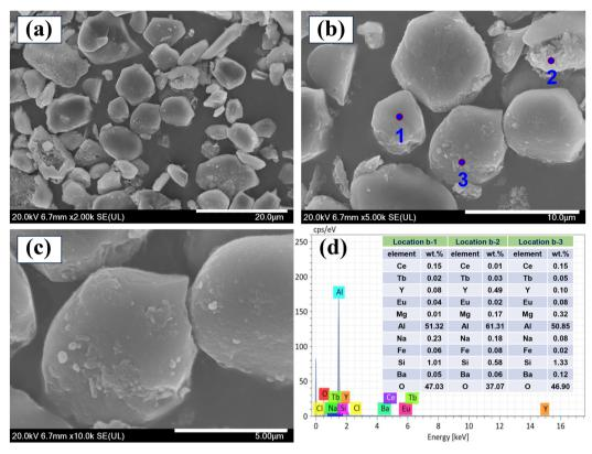
Fig. 5 SEM images of the leaching residue. (a: ×2000; b: ×5000, c: ×10000), and (d) EDS spectra of the leaching residue. (Points 1, 2, and 3 from b).
