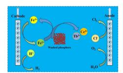
Fig. 6 Schematic diagram of electrochemical reduction leaching mechanism.
