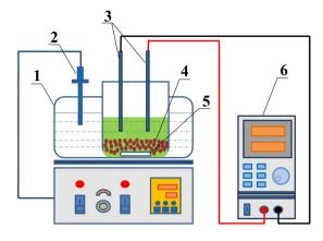
1. Water bath; 2. Thermocouple; 3. Electrodes; 4. Magnetic rotor; 5. Washed phosphor; 6. DC
