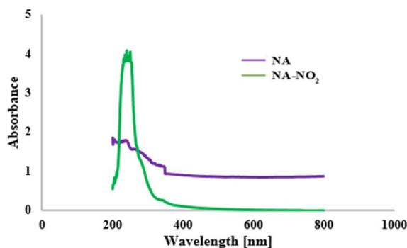
Fig. 5 UV-visible absorption spectra for NA and NA-NO<sub>2</sub>.
