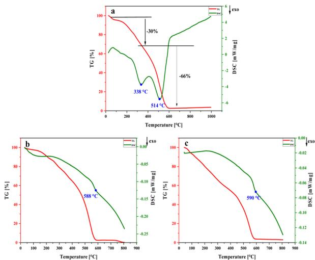
Fig. 11 TG-DSC curves of NA-NO<sub>2</sub> (a), PP-NO<sub>2</sub> (b) and PB-NO<sub>2</sub> (c).
