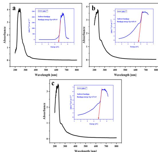
Fig. 10 Indirect band gap energies (a) NA-NO<sub>2</sub>, (b) PP-NO<sub>2</sub> (c) and PB-NO<sub>2</sub>.
