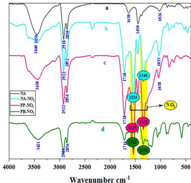
Fig. 4 FTIR spectra of NA (a), NA-NO<sub>2</sub> (b), PP-NO<sub>2</sub> (c) and PB-NO<sub>2</sub> (d).
