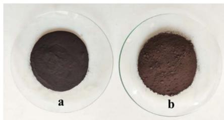
Fig. 2 Color of natural asphalt (a) and NA-NO<sub>2</sub> (b).
