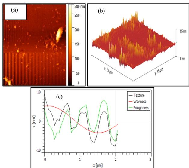
Fig. 9 AFM images of the NA-NO<sub>2</sub>; (a) 2D image, (b) 3D image and (c) texture and roughness analysis.
