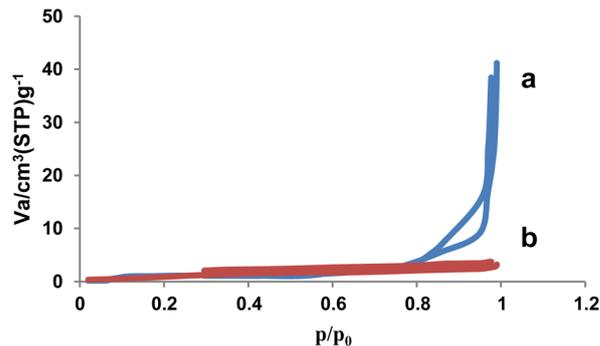
Fig. 6 The N<sub>2</sub> adsorption-desorption isotherm of NA (a) and NA-NO<sub>2</sub> (b).
