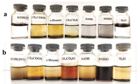
Fig. 1 Solubility of natural asphalt (a) and NA-NO 2 (b).
