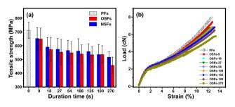
Fig. 5 (a) The tensile strength of OSFs and NSFs as a function of the duration time, and (b) the stress-strain curves of the OSFs samples.
