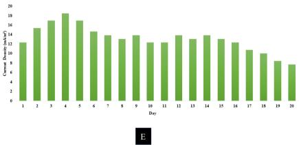
Fig. 4 Bioelectricity generation rate of aannery wastewater: (A) voltage (V), (B) current (mA), (C) power (mW), (D) power density (mW m<sup>-2</sup>), and (E) current density (mA m<sup>-2</sup>) at the Zn-Cu electrode MDC.
