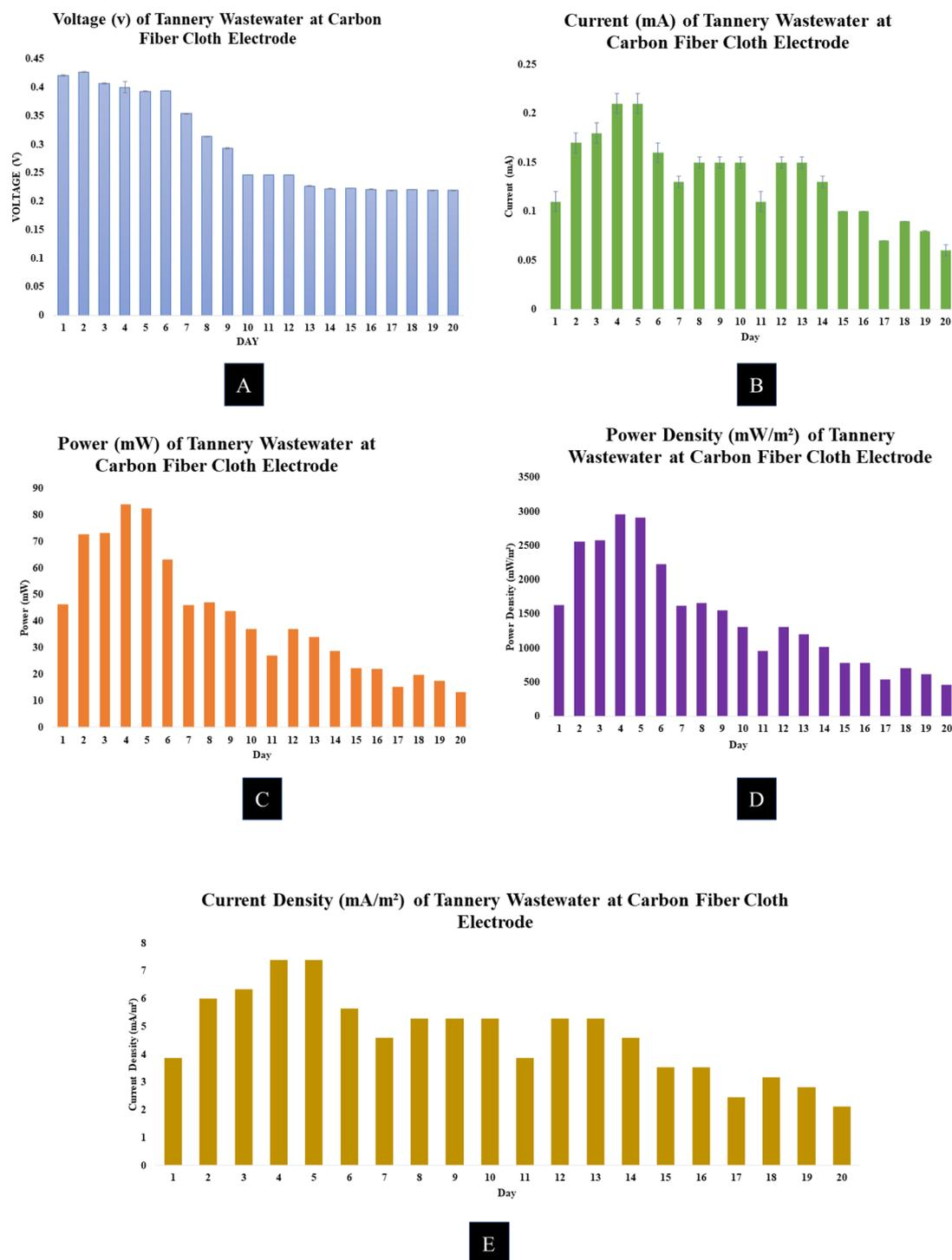
Fig. 5 Bioelectricity generation rate of tannery wastewater: (A) voltage (V), (B) current (mA), (C) power (mW), (D) power density (mW m<sup>-2</sup>), and (E) current density (mA m<sup>-2</sup>) at the carbon fiber cloth electrode MDC.
