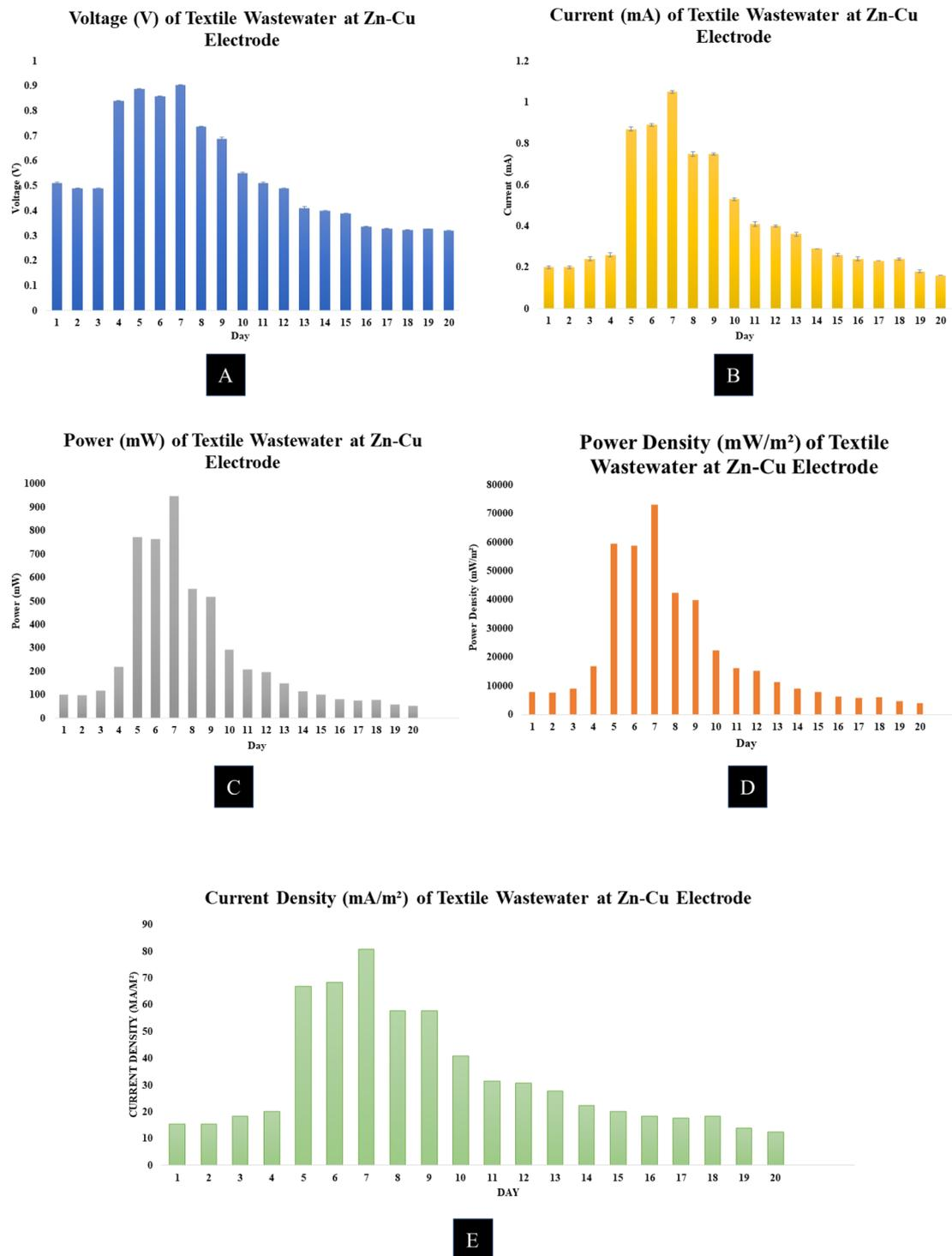
Fig. 2 Bioelectricity generation rate of textile wastewater: (A) voltage (V), (B) current (mA), (C) power (mW), (D) power density (mW m<sup>-2</sup>), and (E) current density (mA m<sup>-2</sup>) at the Zn-Cu electrode MDC.
