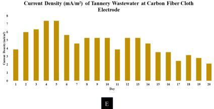
Fig. 5 Bioelectricity generation rate of tannery wastewater: (A) voltage (V), (B) current (mA), (C) power (mW), (D) power density (mW  $m^{-2}$ ), and (E) current density (mA  $m^{-2}$ ) at the carbon fiber cloth electrode MDC.
