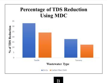
Fig. 6 (A) Percentage of the COD removal rate from wastewater using an MDC and (B) percentage of TDS reduction from wastewater using an MDC.
