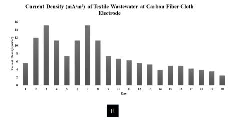
Fig. 3 Bioelectricity generation rate of textile wastewater: (A) voltage (V), (B) current (mA), (C) power (mW), (D) power density (mW m $^{-2}$ ), and (E) current density (mA m $^{-2}$ ) at the carbon fiber cloth electrode MDC.
