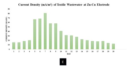
Fig. 2 Bioelectricity generation rate of textile wastewater: (A) voltage (V), (B) current (mA), (C) power (mW), (D) power density (mW m<sup>-2</sup>), and (E) current density (mA m<sup>-2</sup>) at the Zn-Cu electrode MDC.
