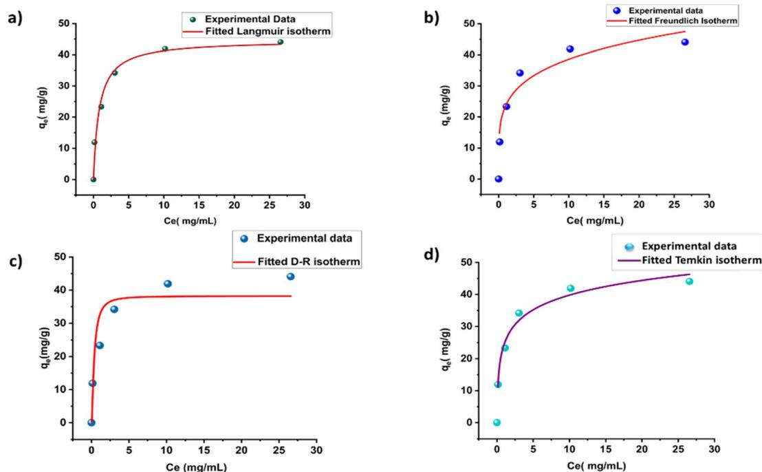
Fig. 10 Non-linear fit Langmuir isotherm (a); non-linear fit Freundlich isotherm (b); non-linear fit D-R isotherm (c) and non-linear fit Temkin isotherm (d) for the adsorption of Malachite Green (pH = 7, dose = 50 mg, time = 90 min).
