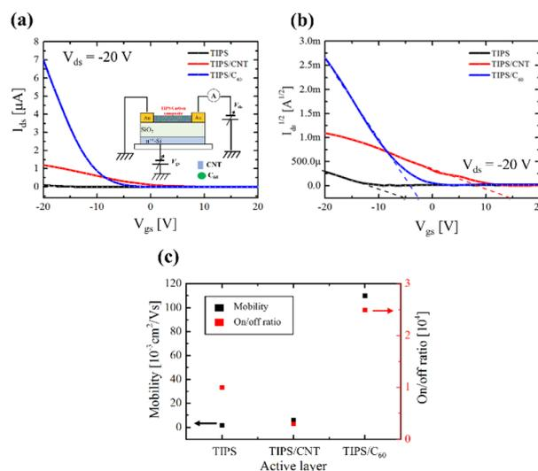
Fig. 6 (a)  $I_{ds}-V_{gs}$  characteristics for TIPS/carbon composite FET with the concentration of 0.1 wt%. (b) Replots for  $\sqrt{I_{ds}-V_{gs}}$  and (c) comparison of performance parameter in TIPS/carbon materials composite. The inset image indicates the schematic representation of TIPS/carbon composite FET structure.
