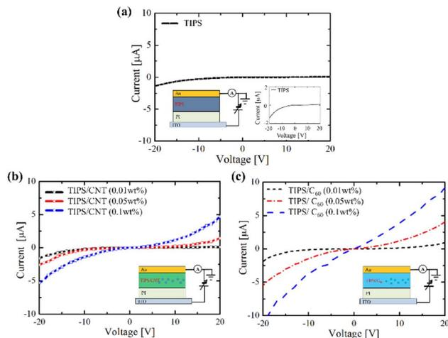
Fig. 1 *I*-*V* characteristics of (a) TIPS, (b) TIPS/CNT composite, and (c) TIPS/C<sub>60</sub> composite diodes with a concentration of 0.01, 0.05, and 0.1 wt%, respectively. The inset images indicate the schematic representation of each device and enlarged image.
