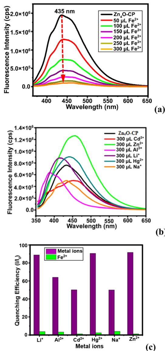
Fig. 5 (a) The fluorescence emission of a solution of the zinc-coordination polymer (3 mL suspension of 4 mg  $\text{Zn}_4\text{O-CP}$  in 10 mL DMF sonicated for 10 min) after each addition of  $\text{Fe}^{2+}$  ions (50  $\mu\text{L}$  of 10 mM aqueous). (b) The effect of different metal ions on the emission spectra of the  $\text{Zn}_4\text{O-CP}$ . (c) Bar-graph of relative quenching caused by  $\text{Fe}^{2+}$  ions as compared to various other metal ions.
