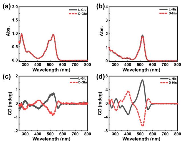
Fig. 4 (a) UV-vis absorption and (c) CD spectra of the mixture of  $1.0 \times 10^{-3}$  M R-C in  $\text{CH}_3\text{CN}$  and  $1.0 \times 10^{-3}$  M L-Glu or D-Glu in deionized water, respectively. (b) UV-vis absorption and (d) CD spectra of the mixture of  $1.0 \times 10^{-3}$  M R-C in  $\text{CH}_3\text{CN}$  and  $1.0 \times 10^{-3}$  M L-His or D-His in deionized water, respectively. ( $d = 2$  mm).
