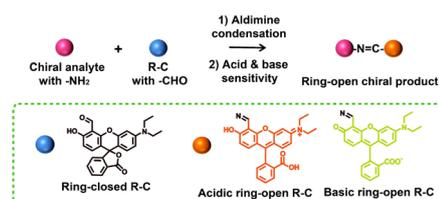
Scheme 1 Schematic diagram of the chiral detection mechanism between R–C and the chiral molecules with –NH<sub>2</sub>.
