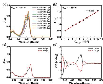
Fig. 2 (a) UV-vis absorption spectra and (b) corresponding absorption values at 522 nm of the mixture of  $1.0 \times 10^{-3}$  M R-C in  $\text{CH}_3\text{CN}$  and L-Cys with various concentrations in deionized water. (c) UV-vis absorption and (d) CD spectra of the mixture of  $1.0 \times 10^{-3}$  M R-C in  $\text{CH}_3\text{CN}$  and  $1.0 \times 10^{-3}$  M L-Cys or D-Cys in deionized water, respectively. ( $d = 2$  mm).
