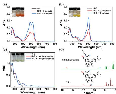
Fig. 1 UV-vis absorption spectra of  $1.0 \times 10^{-4}$  M R-C in  $\text{CH}_3\text{CN}$  and when it was mixed with various eq. (a) acid (TFA), (b) base (TBAOH), and (c) butylamine (BA), respectively. Inset pictures: corresponding photographs of these functional solutions. ( $d = 1$  cm) (d)  $^1\text{H}$  NMR spectra of R-C and the mixture of R-C with BA in deuterated dimethyl sulfoxide (DMSO).
