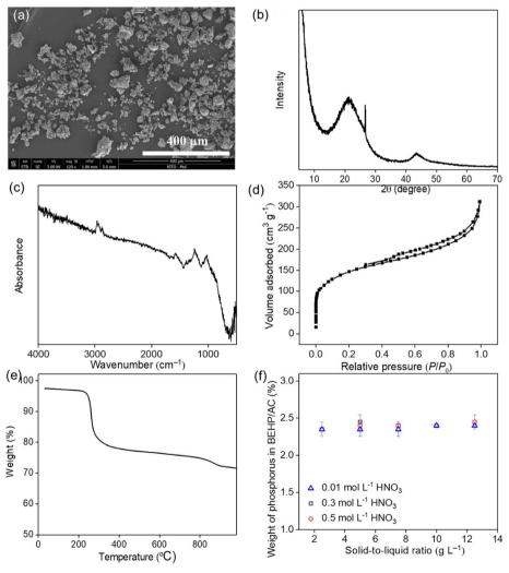
Fig. 1 SEM image (a), XRD pattern (b), FT-IR spectrum (c), N<sub>2</sub> sorption curve (d), TGA curve (e), and phosphorus leaching (f) of HDEHP/AC.
