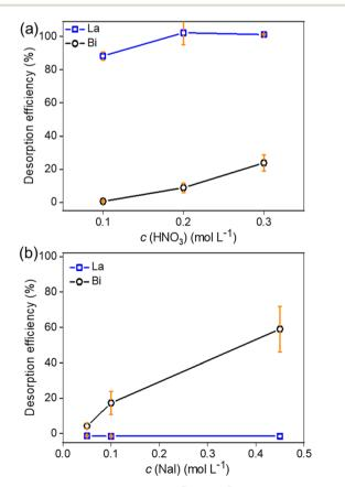
Fig. 9 The desorption efficiency of  $La^{3+}$  and  $Bi^{3+}$  from the HDEHP/AC as of function of  $HNO_3$  (a) concentration and Nal concentration (pH = 2) (b).
