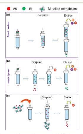
Fig. 10 Conceptual separation process of the direct generator (a), inverse generator (b), and a possible method (c).
