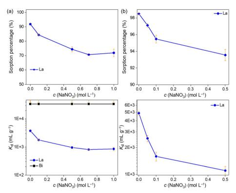
Fig. 3 Effect of NaNO<sub>3</sub> concentration on the sorption performance of HDEHP for La<sup>3+</sup> and Bi<sup>3+</sup> in the binary system with a solid-to-liquid ratio of 3 (a) or 13.3 g L<sup>-1</sup> (b). ( $C_o$  (La<sup>3+</sup>) = 10  $\mu$ mol L<sup>-1</sup> and  $C_o$  (Bi<sup>3+</sup>) = 10  $\mu$ mol L<sup>-1</sup>, pH = 2, t = 24 h).
