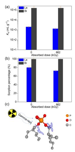
Fig. 7 Effect of absorbed dose on the distribution coefficient (a) and sorption percentage ( $K_d$ ) (b) of HDEHP/AC for La<sup>3+</sup> and Bi<sup>3+</sup> in the binary system. ( $C_o$  (La<sup>3+</sup>) = 10  $\mu$ mol L<sup>-1</sup> and  $C_o$  (Bi<sup>3+</sup>) = 10  $\mu$ mol L<sup>-1</sup> solid-to-liquid ratio = 2 g L<sup>-1</sup>, pH = 2, t = 24 h). Schematic illustration of scission of functional groups by gamma irradiation (c).
