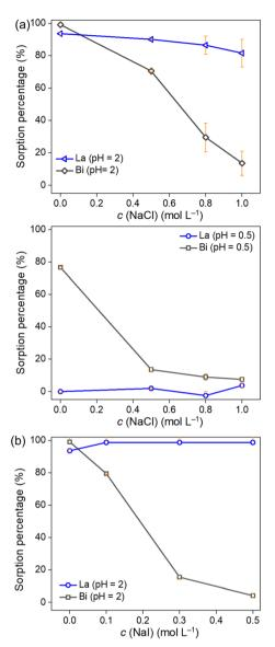
Fig. 4 Effect of NaCl (a) and Nal (b) concentration on the sorption performance of HDEHP for La $^{3+}$  and Bi $^{3+}$  in the binary system. ( $C_{\rm o}$  (La $^{3+})=10~\mu{\rm mol}~{\rm L}^{-1}$  and  $C_{\rm o}$  (Bi $^{3+})=10~\mu{\rm mol}~{\rm L}^{-1}$ , solid-to-liquid ratio  $=13.3~{\rm g}~{\rm L}^{-1},~t=24~{\rm h}).$
