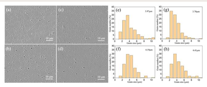
Fig. 3 SEM micrographs of the polished and thermally etched surfaces of  $Sr_{4-x}La_xNa_2Hf_xNb_{10-x}O_{30}$  ceramics: (a) x = 0, (b) x = 0.2, (c) x = 0.4, (d) x = 0.6. The grain size distribution of the samples corresponding to (a–d): (e) x = 0, (f) x = 0.2, (g) x = 0.4, (h) x = 0.6.
