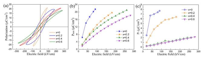
Fig. 7 (a) Polarization-electric field (P-E) curve measured at ambient temperature with a triangular wave form at 10 Hz for  $Sr_{4-x}La_xNa_2Hf_xNb_{10-x}O_{30}\ ceramics;\ (b)\ the\ variation\ in\ P_{max}\ with\ increasing\ imposed\ electric\ field\ for\ Sr_{4-x}La_xNa_2Hf_xNb_{10-x}O_{30}\ ceramics;\ (c)\ the\ property of the property of the$ variation in  $P_r$  with increasing imposed electric field for  $Sr_{4-x}La_xNa_2Hf_xNb_{10-x}O_{30}$  ceramics.
