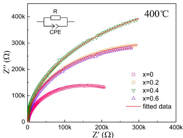
Fig. 5 Complex impedance spectrum at  $400\text{ }^\circ\text{C}$  for  $\text{Sr}_{4-x}\text{La}_x\text{Na}_2\text{Hf}_x\text{Nb}_{10-x}\text{O}_{30}$  ( $x = 0, 0.2, 0.4$  and  $0.6$ ) ceramics. The red line indicates the fitted data. The inset shows the equivalent circuit diagram of the impedance data.
