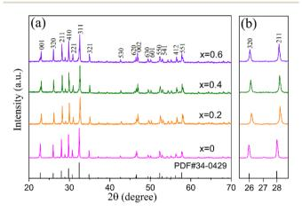
Fig. 1 (a) XRD patterns of  $Sr_{4-x}La_xNa_2Hf_xNb_{10-x}O_{30}$  (x=0, 0.2, 0.4 and 0.6) ceramics; (b) partial enlargement drawing of diffraction peaks of (320) and (211).
