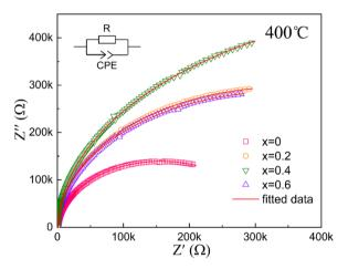
Fig. 5 Complex impedance spectrum at 400 °C for  $Sr_{4-x}La_xNa_2Hf_xNb_{10-x}O_{30}$  (x=0, 0.2, 0.4 and 0.6) ceramics. The red line indicates the fitted data. The inset shows the equivalent circuit diagram of the impedance data.
