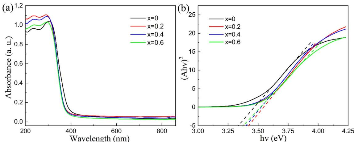
Fig. 4 (a) UV-vis absorption spectrum for  $\text{Sr}_{4-x}\text{La}_x\text{Na}_2\text{Hf}_x\text{Nb}_{10-x}\text{O}_{30}$  ( $x = 0, 0.2, 0.4$  and  $0.6$ ); (b)  $(Ah\nu)^2$  vs.  $h\nu$  plots for  $\text{Sr}_{4-x}\text{La}_x\text{Na}_2\text{Hf}_x\text{Nb}_{10-x}\text{O}_{30}$  ( $x = 0, 0.2, 0.4$  and  $0.6$ ).
