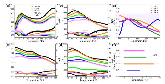
Fig. 6 Temperature dependences of dielectric permittivity  $\varepsilon_r$  and dielectric loss  $\tan\delta$  for  $\mathrm{Sr}_{4-x}\mathrm{La}_x\mathrm{Na}_2\mathrm{Hf}_x\mathrm{Nb}_{10-x}\mathrm{O}_{30}$  ceramics: (a) x=0, (b) x=0.2, (c) x = 0.4, (d) x = 0.6; (e) evolution of  $\Delta \varepsilon / \varepsilon_0 \circ_C (\Delta \varepsilon = \varepsilon_r - \varepsilon_0 \circ_C)$  as a function of temperature for SSNFN ceramic at 10 kHz; (f) temperature range of
