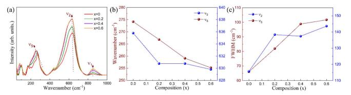
Fig. 2 (a) Raman spectra for  $Sr_{4-x}La_xNa_2Hf_xNb_{10-x}O_{30}$  (x=0, 0.2, 0.4 and 0.6) ceramics at ambient temperature; (b) Raman shift of the  $\nu_2$  and  $\nu_5$  modes; (c) full width at half maximum (FWHM) of the  $\nu_2$  and  $\nu_5$  modes.
