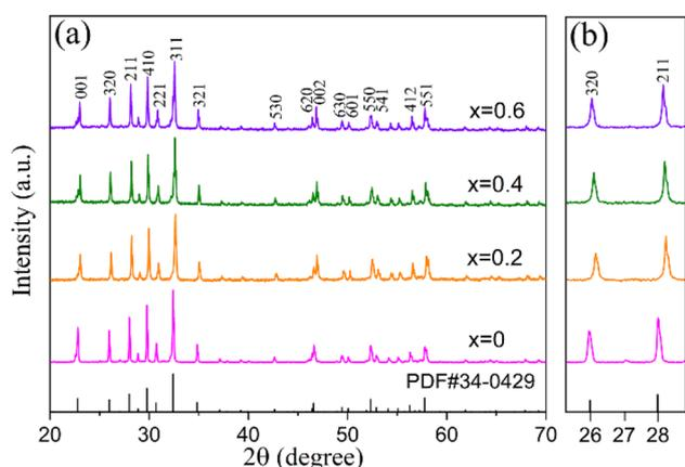
Fig. 1 (a) XRD patterns of  $\text{Sr}_{4-x}\text{La}_x\text{Na}_2\text{Hf}_x\text{Nb}_{10-x}\text{O}_{30}$  ( $x = 0, 0.2, 0.4$  and  $0.6$ ) ceramics; (b) partial enlargement drawing of diffraction peaks of (320) and (211).
