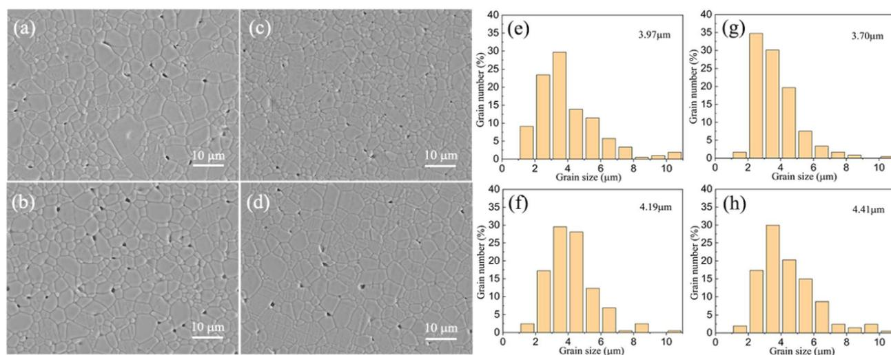
Fig. 3 SEM micrographs of the polished and thermally etched surfaces of  $\text{Sr}_{4-x}\text{La}_x\text{Na}_2\text{Hf}_x\text{Nb}_{10-x}\text{O}_{30}$  ceramics: (a)  $x = 0$ , (b)  $x = 0.2$ , (c)  $x = 0.4$ , (d)  $x = 0.6$ . The grain size distribution of the samples corresponding to (a)–(d): (e)  $x = 0$ , (f)  $x = 0.2$ , (g)  $x = 0.4$ , (h)  $x = 0.6$ .
