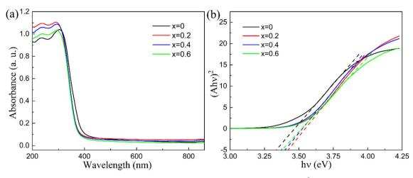
Fig. 4 (a) UV-vis absorption spectrum for  $Sr_{4-x}La_xNa_2Hf_xNb_{10-x}O_{30}$  (x=0, 0.2, 0.4 and 0.6); (b)  $(Ahv)^2$  vs. hv plots for  $Sr_{4-x}La_xNa_2Hf_xNb_{10-x}O_{30}$  (x=0, 0.2, 0.4 and 0.6).
