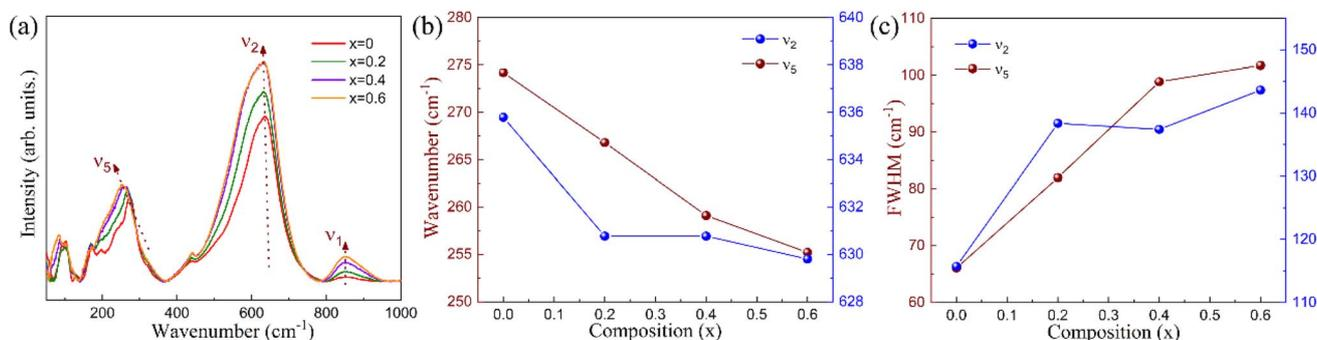
Fig. 2 (a) Raman spectra for  $\text{Sr}_{4-x}\text{La}_x\text{Na}_2\text{Hf}_x\text{Nb}_{10-x}\text{O}_{30}$  ( $x = 0, 0.2, 0.4$  and  $0.6$ ) ceramics at ambient temperature; (b) Raman shift of the  $\nu_2$  and  $\nu_5$  modes; (c) full width at half maximum (FWHM) of the  $\nu_2$  and  $\nu_5$  modes.
