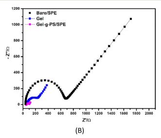
Fig. 4 Electrochemical characterization. (A) Cyclic voltammetry curves and (B) electrochemical impedance spectroscopy (EIS) of bare (unmodified)/SPE, Gel/SPE and Gel-g-PS/SPE in a mixture solution of 5 mM of FCN redox probe and 0.1 M of KCl at scan rate of 50 mV s<sup>-1</sup>.
