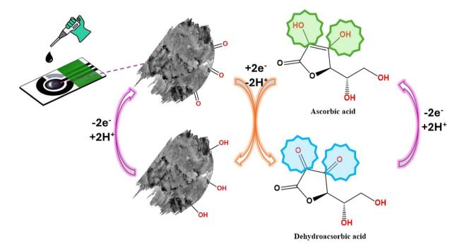
Fig. 7 The schematic diagram showed the preparation and sensing response of Gel-g-PS -modified screen-printed electrode toward ascorbic acid detection.
