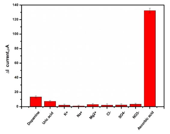
Fig. 9 Interference study of the proposed sensor (Gel-g-PS/SPE) toward 60 ppb ascorbic acid and 120 ppb of uric acid, dopamine, K<sup>+</sup>, Na<sup>+</sup>,  $Mg^{2+}$ ,  $Cl^-$ ,  $SO^{4-}$ , and  $NO^{3-}$  in PBS (pH 7.4). The experiments for each interferent were conducted in triplicate.
