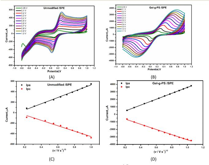
Fig. 5 Oxidation and reduction peak currents of solution containing 5 mM [Fe(CN) $_6$ ] $^{4-/3-}$  and 0.1 M of KCl at different scan rates for (A) bare SPE (unmodified SPE) and (B) Gel-g-PS/SPE. Ipa and Ipc linearity lines corresponding to CVs for (C) bare, and (D) Gel-g-PS/SPE recorded at different scan rates.
