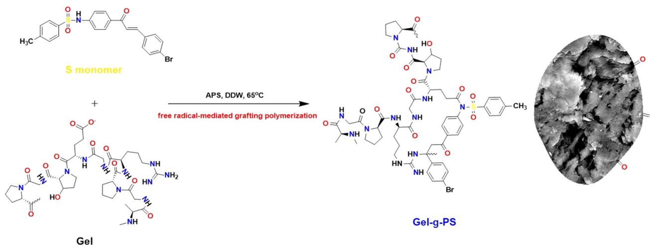
Fig. 1 The schematic representation of Gel-g-PS formation.
