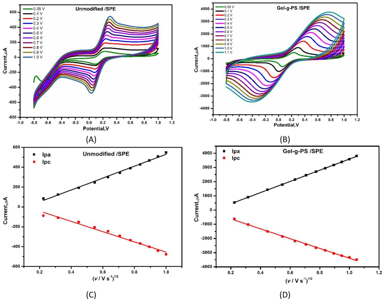
Fig. 5 Oxidation and reduction peak currents of solution containing 5 mM  $[\text{Fe}(\text{CN})_6]^{4-/3-}$  and 0.1 M of KCl at different scan rates for (A) bare SPE (unmodified SPE) and (B) Gel-g-PS/SPE.  $I_{\text{pa}}$  and  $I_{\text{pc}}$  linearity lines corresponding to CVs for (C) bare, and (D) Gel-g-PS/SPE recorded at different scan rates.
