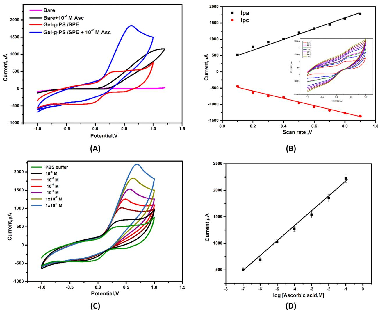
Fig. 6 (A) Cyclic voltammograms of the bare/SPE and Gel-g-PS/SPE in PBS (pH 7.4) in the absence and present  $10^{-2} \text{ M}$  of ascorbic acid. (B) Scan rate effect of Gel-g-PS/SPE. (C) Cyclic voltammetry curves obtained after addition of different concentrations of ascorbic acid in PBS (pH 7.4). (D) Calibration curve of current vs. log concentration of AA.
