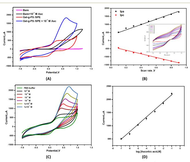
Fig. 6 (A) Cyclic voltammograms of the bare/SPE and Gel-g-PS/SPE in PBS (pH 7.4) in the absence and present 10<sup>-2</sup> M of ascorbic acid. (B) Scan rate effect of Gel-g-PS/SPE. (C) Cyclic voltammetry curves obtained after addition of different concentrations of ascorbic acid in PBS (pH 7.4). (D) Calibration curve of current vs. log concentration of AA.
