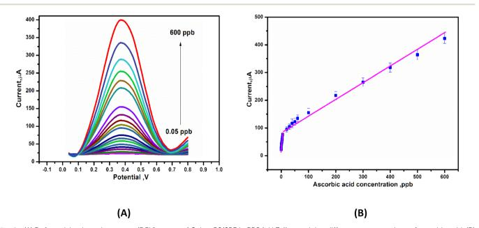
Fig. 8 (A) Deferential pulse voltammetry (DPV) curves of Gel-g-PS/SPE in PBS (pH 7.4) containing different concentrations of ascorbic acid. (B) Calibration curve for ascorbic acid detection obtained from DPV measurements.
