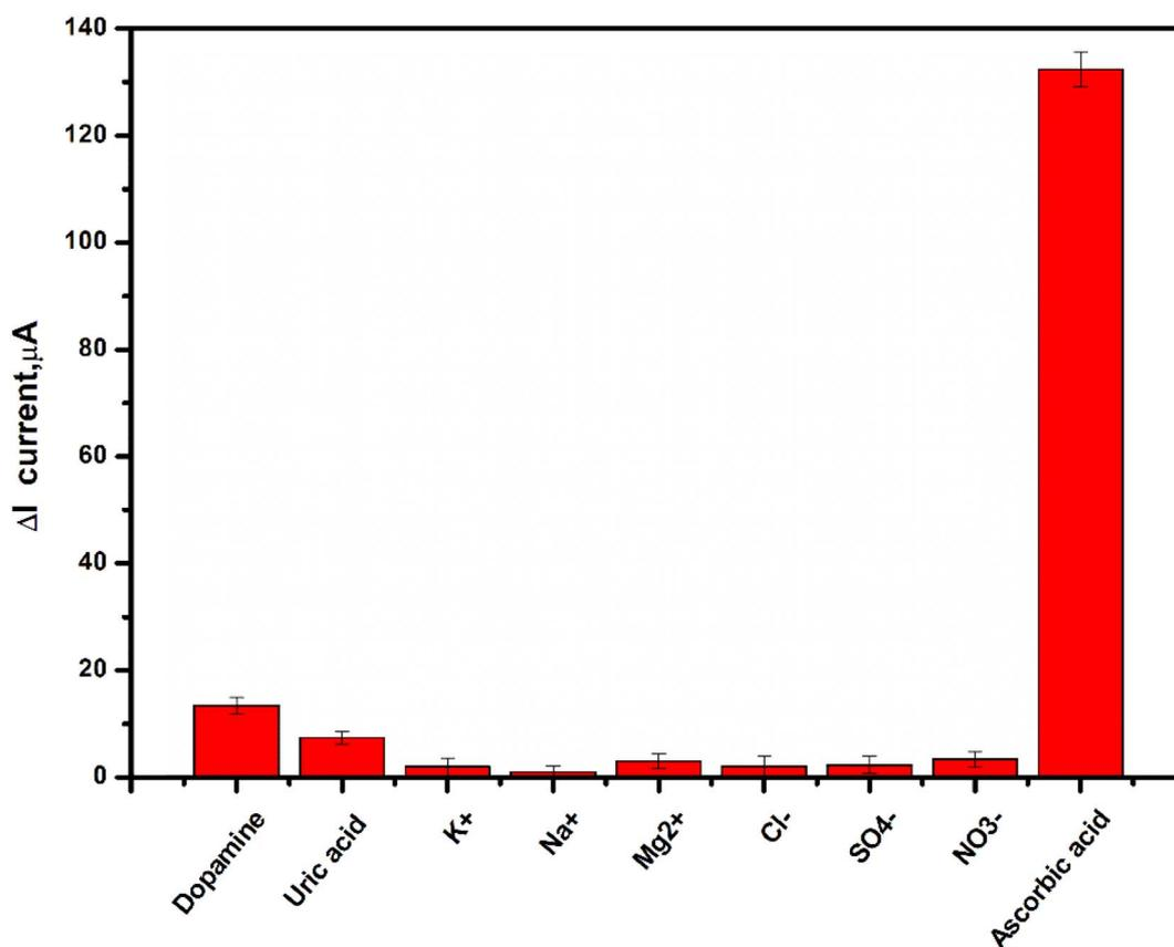
Fig. 9 Interference study of the proposed sensor (Gel-g-PS/SPE) toward 60 ppb ascorbic acid and 120 ppb of uric acid, dopamine, K<sup>+</sup>, Na<sup>+</sup>, Mg<sup>2+</sup>, Cl<sup>-</sup>, SO<sub>4</sub><sup>2-</sup>, and NO<sub>3</sub><sup>-</sup> in PBS (pH 7.4). The experiments for each interferent were conducted in triplicate.
