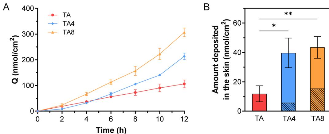
Fig. 4 Skin penetration and deposition of TA and its ester derivatives. (A) Cumulative amount of each compound permeated ( $Q$ ) through porcine skin over 12 h ( $n = 4$ ). (B) Amount of each compound deposited in the skin after skin permeation experiments ( $n = 4$ ). The diagonally lined portion of the bar graph indicates the amount of TA generated from the hydrolysis of TA derivatives in the skin. \* $p < 0.05$ , \*\* $p < 0.01$ .
