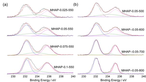
Fig. 3 O 1s XPS spectra of MO<sub>x</sub>/HAP with different Mo loading amounts (a) and calcination temperature (b).
