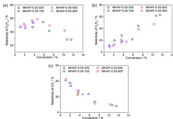
Fig. 10 The selectivity–conversion relationships for cyclohexane ODH over different catalysts. (a) C<sub>6</sub>H<sub>10</sub>, (b) C<sub>6</sub>H<sub>6</sub> and (c) CO<sub>x</sub>.
