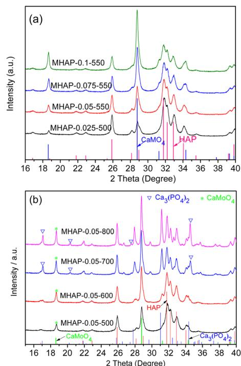
Fig. 1 XRD patterns of HAPs, CaMoO<sub>4</sub>, Ca<sub>3</sub>(PO<sub>4</sub>)<sub>2</sub> and MO<sub>x</sub>/HAP with different MoO<sub>x</sub> loading amounts (a) and calcination temperature (b).
