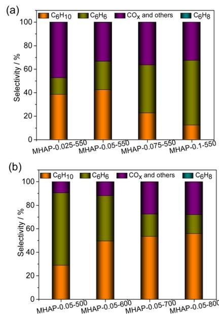
Fig. 9 The product distribution patterns of the MHAP catalysts with different MoO<sub>x</sub> loading amounts (a) and calcination temperature (b).
