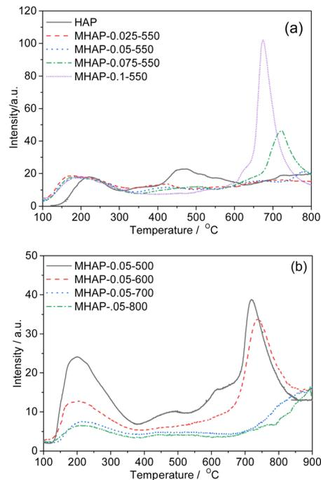
Fig. 7 NH<sub>3</sub>-TPD profiles of MHAP samples with different MoO<sub>x</sub> loading amounts (a) and calcination temperature (b).
