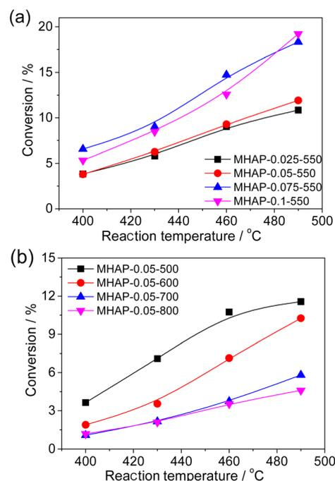
Fig. 8 Catalytic activity of MHAP catalysts with different MoO<sub>x</sub> loading amounts (a) and calcination temperature (b).
