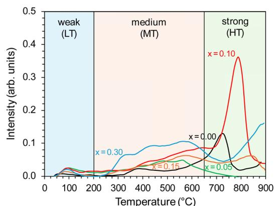
Fig. 2 CO<sub>2</sub>-TPD profiles of the BaCe<sub>1-x</sub>Y<sub>x</sub>O<sub>3-δ</sub> (x = 0–0.30) supports.
