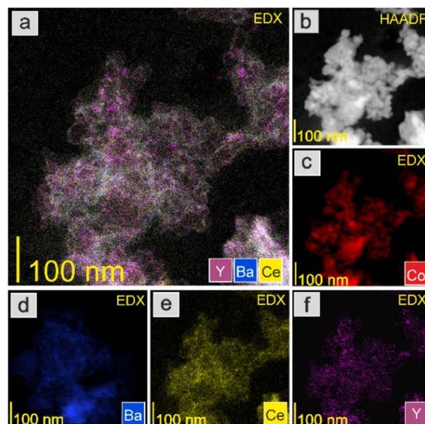
Fig. 9 HAADF-STEM image and EDX maps of the Co/BaCe<sub>1-x</sub>Y<sub>x</sub>O<sub>3- $\delta$</sub>  ( $x = 0.30$ ) catalyst after reduction in hydrogen at 600 °C. (a) Overlay EDX map of Y, Ba, and Ce. (b) HAADF-STEM image. EDX maps of (c) Co, (d) Ba, (e) Ce, and (f) Y.
