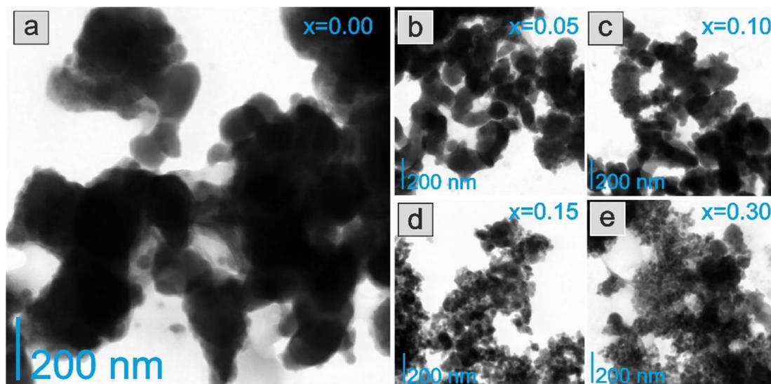
Fig. 4 STEM images of the Co/BaCe<sub>1-x</sub>Y<sub>x</sub>O<sub>3-δ</sub> catalysts after reduction in hydrogen at 600 °C, where (a)  $x = 0$ , (b)  $x = 0.05$ , (c)  $x = 0.10$ , (d)  $x = 0.15$ , (e)  $x = 0.30$ .
