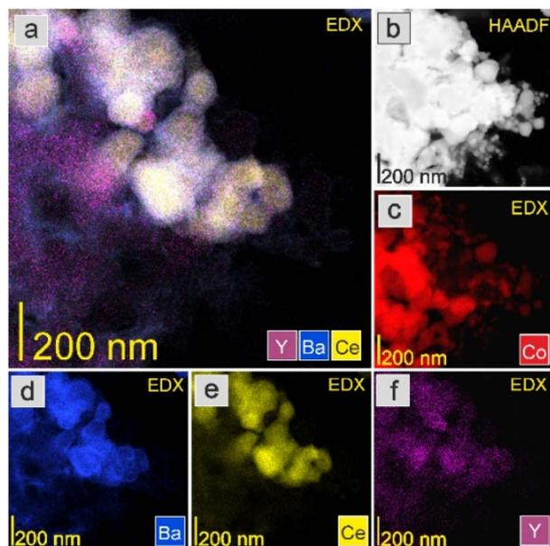
Fig. 6 HAADF-STEM image and EDX maps of the Co/BaCe<sub>1-x</sub>Y<sub>x</sub>O<sub>3- $\delta$</sub>  ( $x = 0.05$ ) catalyst after reduction in hydrogen at 600 °C. (a) Overlay EDX map of Y, Ba, and Ce. (b) HAADF-STEM image. EDX maps of (c) Co, (d) Ba, (e) Ce, and (f) Y.
