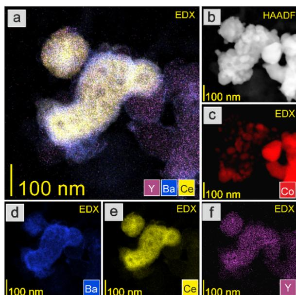
Fig. 7 HAADF-STEM image and EDX maps of the Co/BaCe<sub>1-x</sub>Y<sub>x</sub>O<sub>3- $\delta$</sub>  ( $x = 0.10$ ) catalyst after reduction in hydrogen at 600 °C. (a) Overlay EDX map of Y, Ba, and Ce. (b) HAADF-STEM image. EDX maps of (c) Co, (d) Ba, (e) Ce, and (f) Y.
