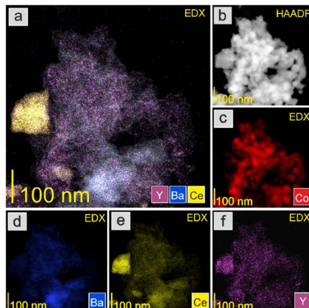
Fig. 8 HAADF-STEM image and EDX maps of the Co/BaCe<sub>1-x</sub>Y<sub>x</sub>O<sub>3- $\delta$</sub>  ( $x = 0.15$ ) catalyst after reduction in hydrogen at 600 °C. (a) Overlay EDX map of Y, Ba, and Ce. (b) HAADF-STEM image. EDX maps of (c) Co, (d) Ba, (e) Ce, and (f) Y.
