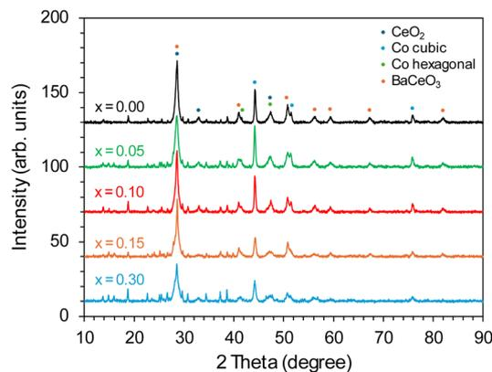
Fig. 3 PXRD patterns of the Co/BaCe<sub>1-x</sub>Y<sub>x</sub>O<sub>3-δ</sub> ( $x = 0-0.30$ ) catalysts after reduction in hydrogen at 600 °C.
