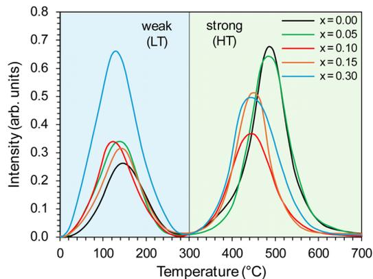
Fig. 11 H<sub>2</sub>-TPD profiles of the Co/BaCe<sub>1-x</sub>Y<sub>x</sub>O<sub>3-δ</sub> ( $x = 0-0.30$ ) catalysts.
