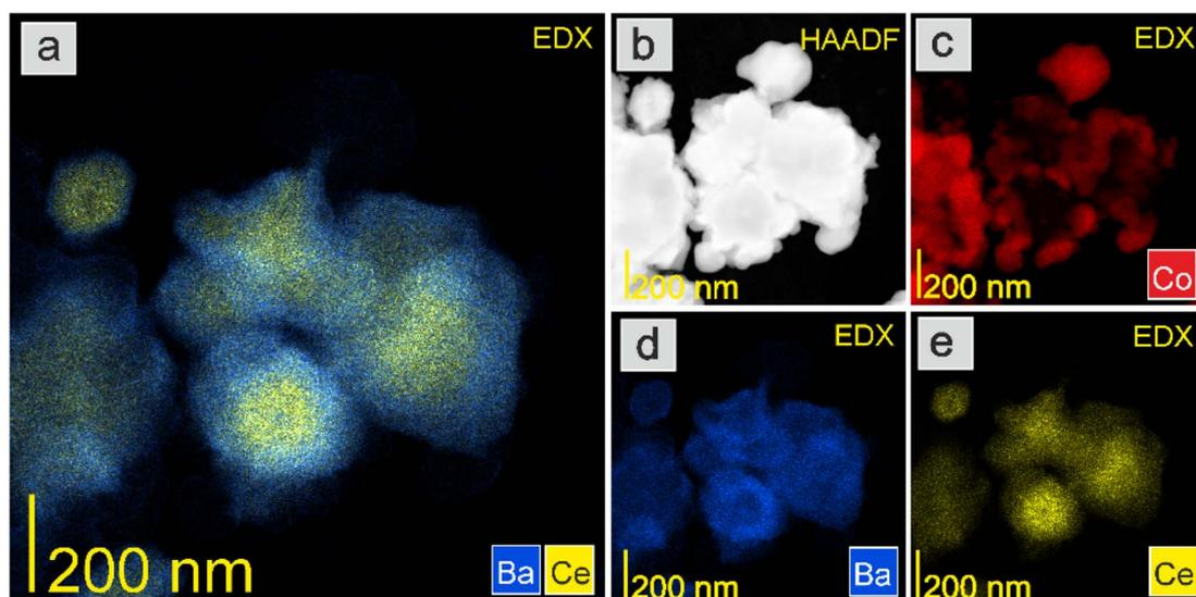
Fig. 5 HAADF-STEM image and EDX maps of the Co/BaCe<sub>1-x</sub>Y<sub>x</sub>O<sub>3-δ</sub> ( $x = 0$ ) catalyst after reduction in hydrogen at 600 °C. (a) Overlay EDX map of Ba and Ce. (b) HAADF-STEM image. EDX maps of (c) Co, (d) Ba, and (e) Ce.
