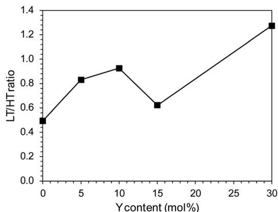
Fig. 12 Low temperature (LT) to high temperature (HT) hydrogen desorption peak ratio of the Co/BaCe<sub>1-x</sub>Y<sub>x</sub>O<sub>3-δ</sub> ( $x = 0-0.30$ ) catalysts.
