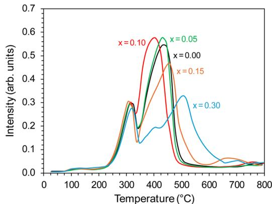
Fig. 10 H<sub>2</sub>-TPR profiles of the Co/BaCe<sub>1-x</sub>Y<sub>x</sub>O<sub>3-δ</sub> ( $x = 0-0.30$ ) catalysts.
